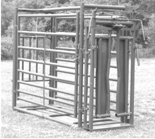
Figure 15 Cattle Chute designed for restricting cattle, credit:ranchcity.com
