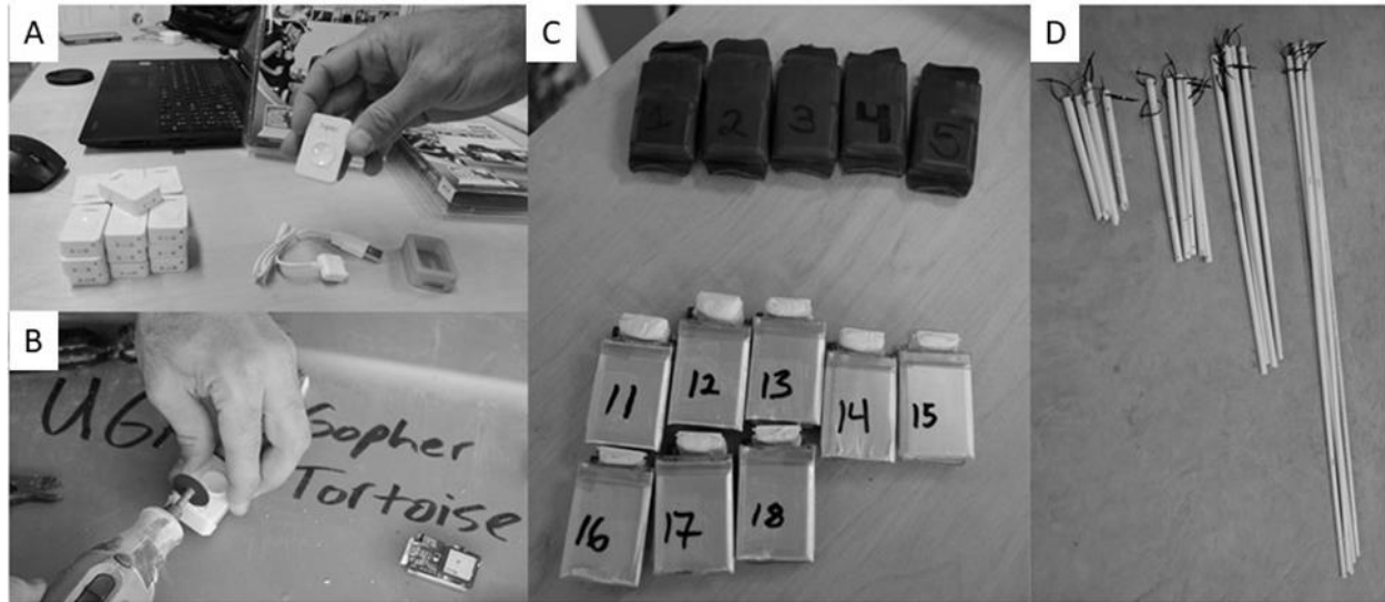
Figure 2.1. A. Mobile Action i-GotU GT-120 GPS loggers. B. Using Dremel equipped with Heavy Duty Cut-Off Wheel to remove the plastic housing on GPS logger. C. Modified and numbered stationary GPS loggers (water-proofed with 3M heat-shrink tubing on top, USB connection ports reinforced with WaterWeld at bottom). D. 20 PVC pipe segments (5 each of 30cm, 50cm, 1m, and 2m long) corresponding to 0.0m, 0.5m, 1.0m, and 2.0m inside burrow locations.
