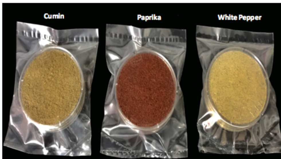
Figure 7.1. Samples in sealed small petri dishes before subjected to RF heating
