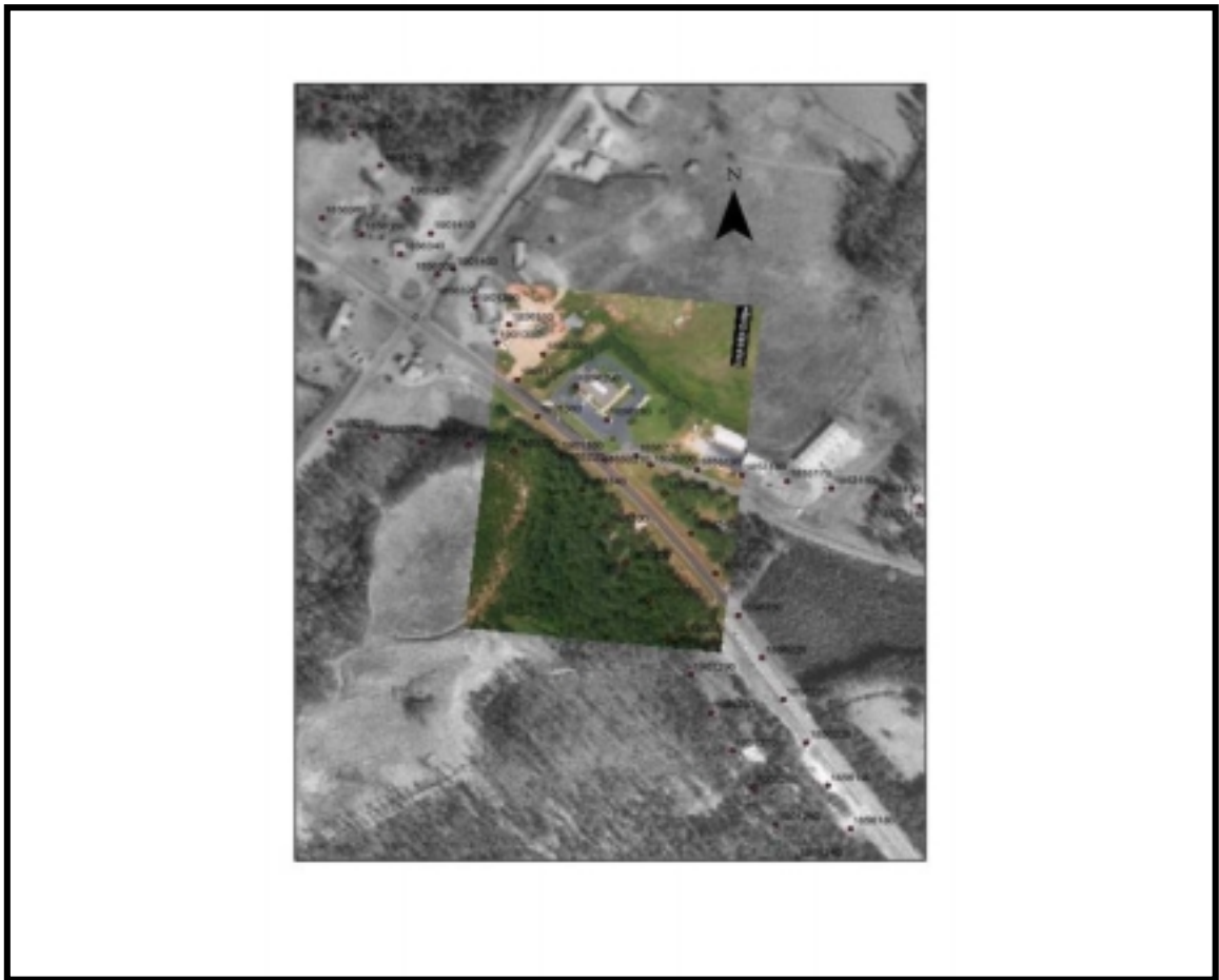
Figure 4.4: Digital Frame Georeferenced on DOQQ with eRTK-Exposure Stations 26-kilometer Baseline.
