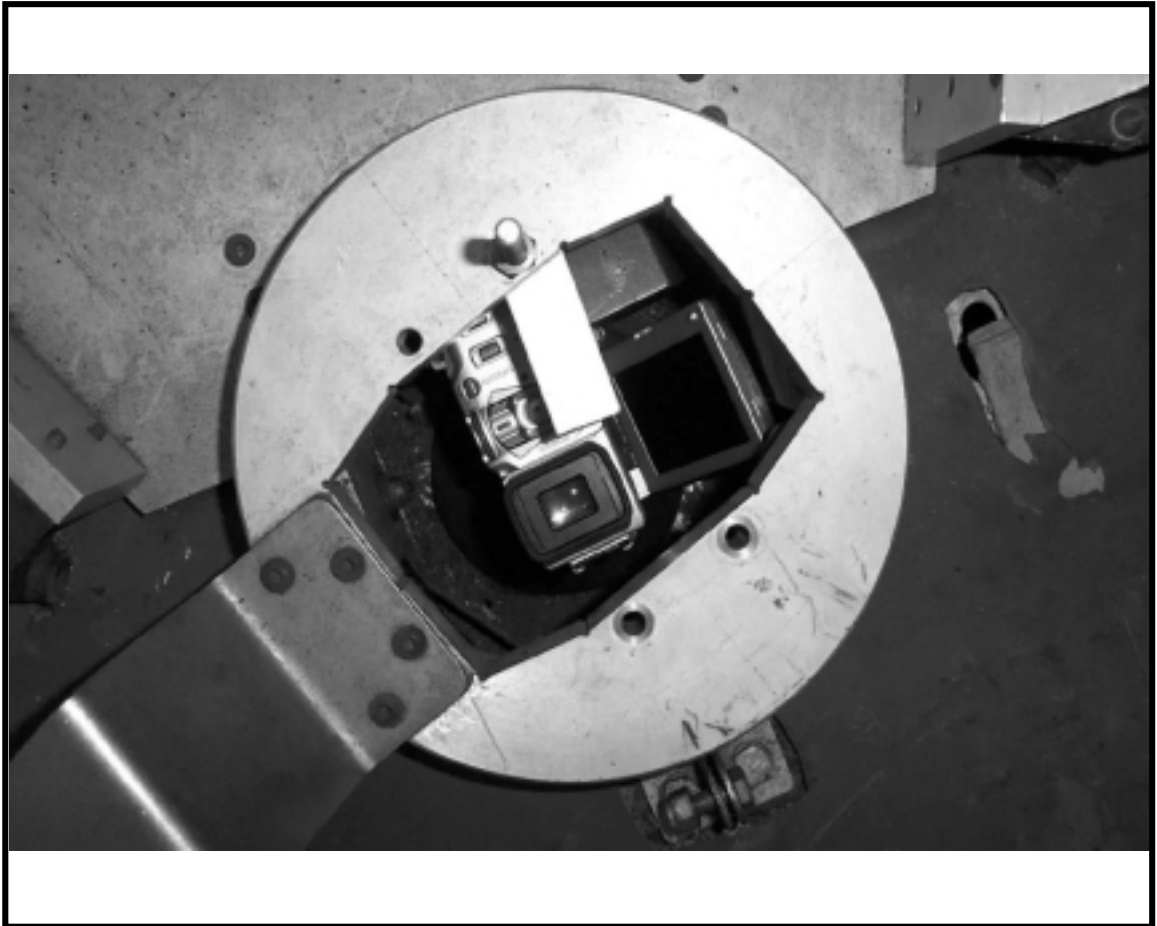
Figure 5.8: SONY PC 1 Digital Frame Video Mounting in Aircraft.
