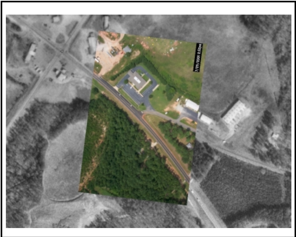
Figure 3.8: Direct Georeferenced Digital Frame Image with eRTK GPS Solution.
