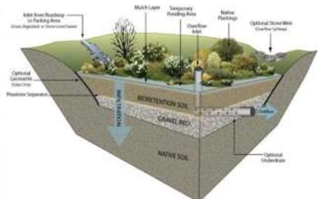
Figure 93. The bioretention (Omaha By Design n.d.) and its structure (Douglas County's Environmental Information Center n.d.)
