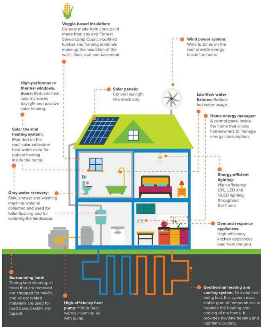
Figure 96. The operation system of a green building (Inhabitat n.d.)
