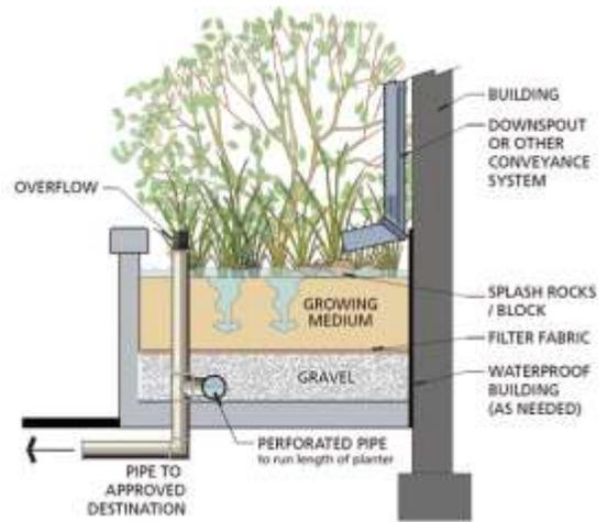
Figure 92. The infiltration planter (Meliora Design n.d.) and its structure (City of Portland n.d.)
