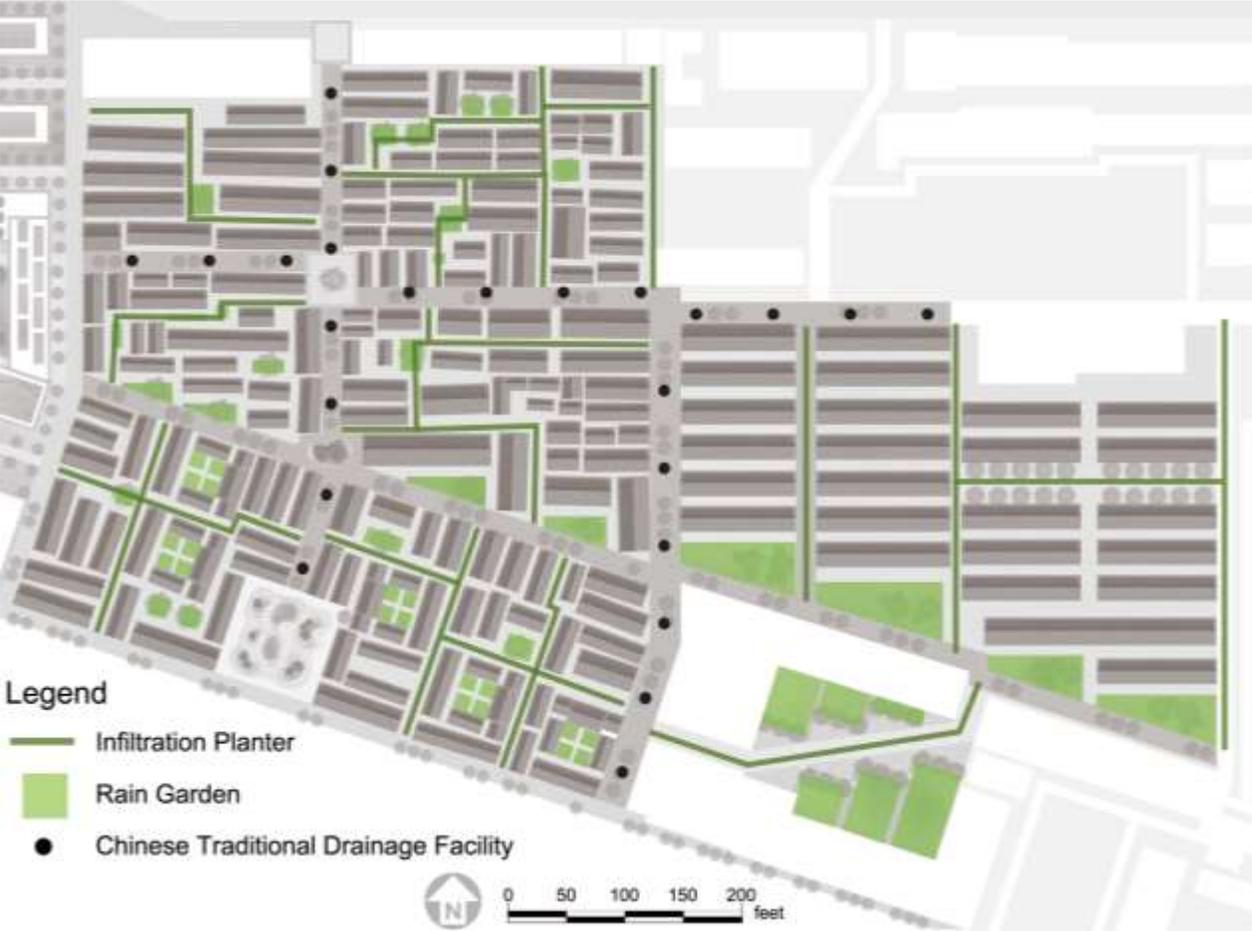
Figure 84. The distribution of drainage facilities
