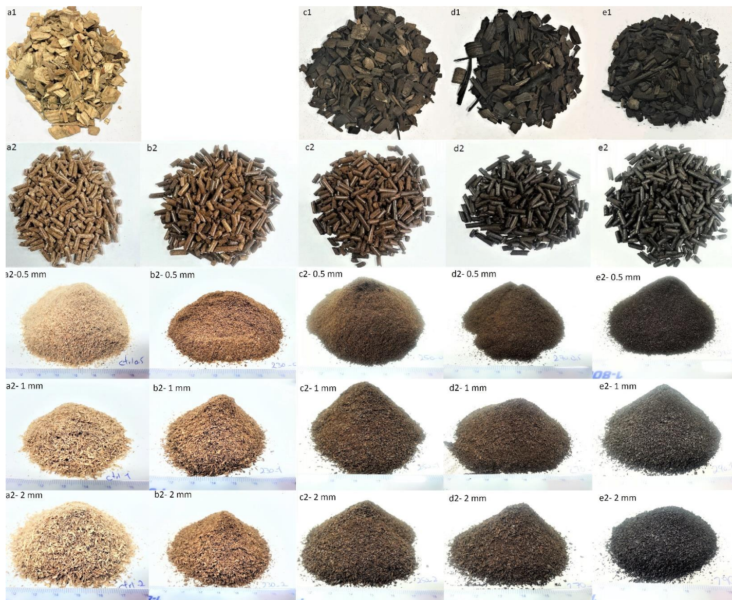
Figure 4-2. Wood chips, wood pellets and ground samples of wood pellets through screens sizes of 2 mm, 1 mm, and 0.5 mm, a) untreated, (b) T230, (c1) T250, d) T270, e) T290. The torrefied wood chips at 230 were not provided.
