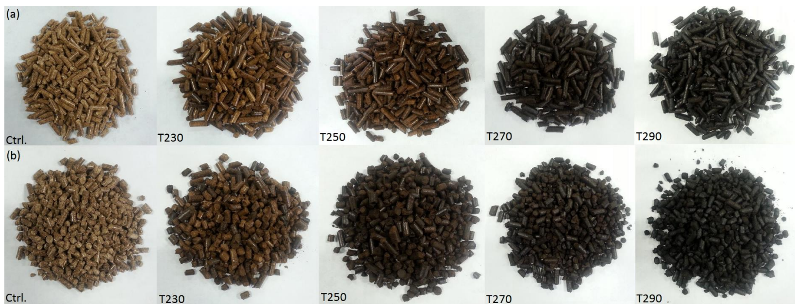
Figure 3-1. Control and torrefied pellets at different torrefaction temperature; (a) CP1 pellets, (b) CP2 pellets. T#: Torrefied at #°C. e.g., T230: torrefied at 230°C.
