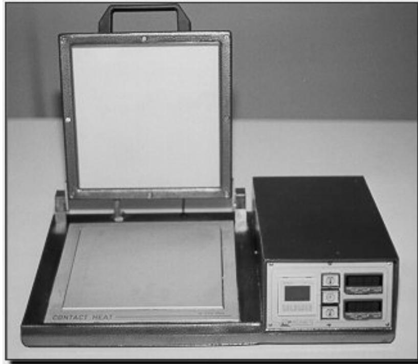
Figure 7. Photograph of Thermo-fixation Apparatus [56].
