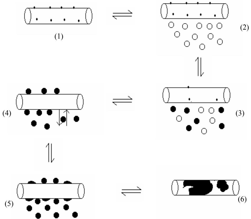
Figure 3. Schematic Representation of Dye-Surfactant Interaction in Polyester High-Temperature Dyeing [44].
