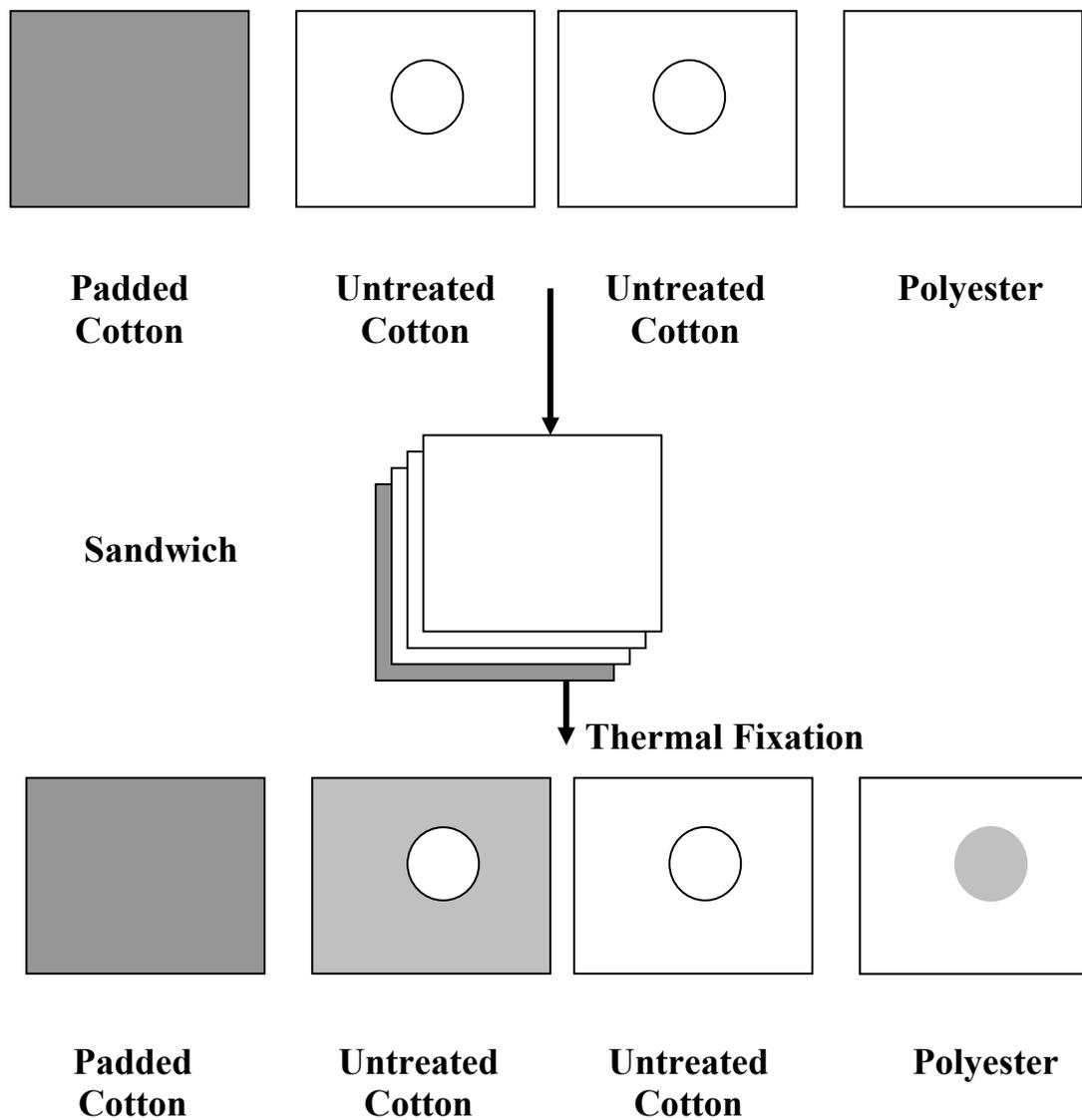
Figure 8. Schematic Representation of Experiment for Measuring Extent of Dye Vaporization.
