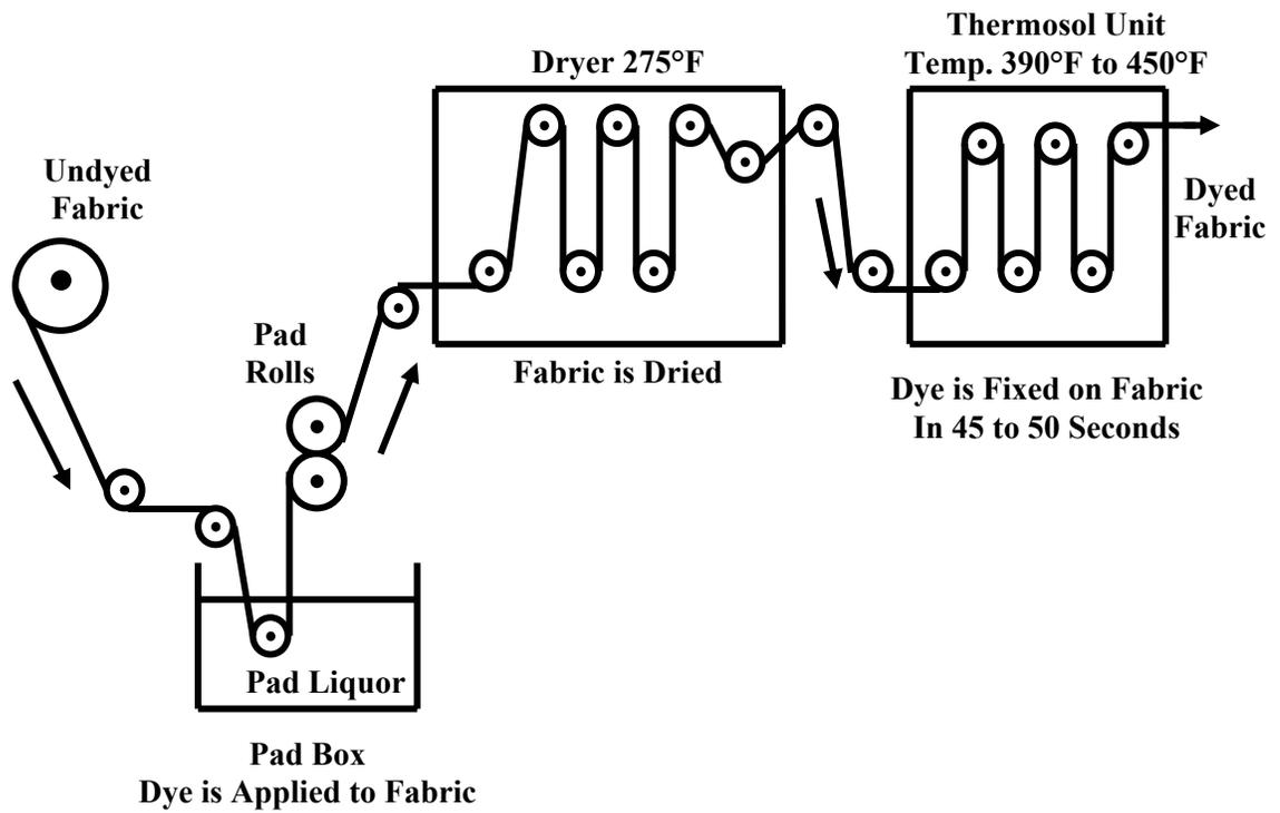
Figure 1. Schematic Representation of the Thermosol Process [8].
