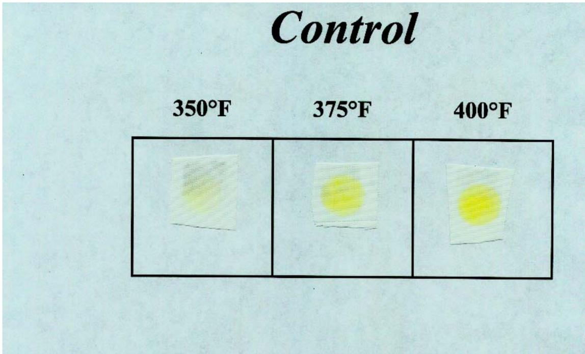
Figure 47. C.I. Disperse Yellow 42 Vaporization in Control Samples.
