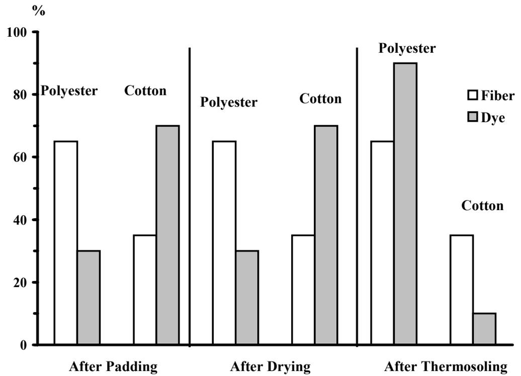
Figure 2. Schematic Representation of Disperse Dye Distribution on 65/35 Polyester/Cotton Fabric at Various Stages of the Thermosol Process [21].
