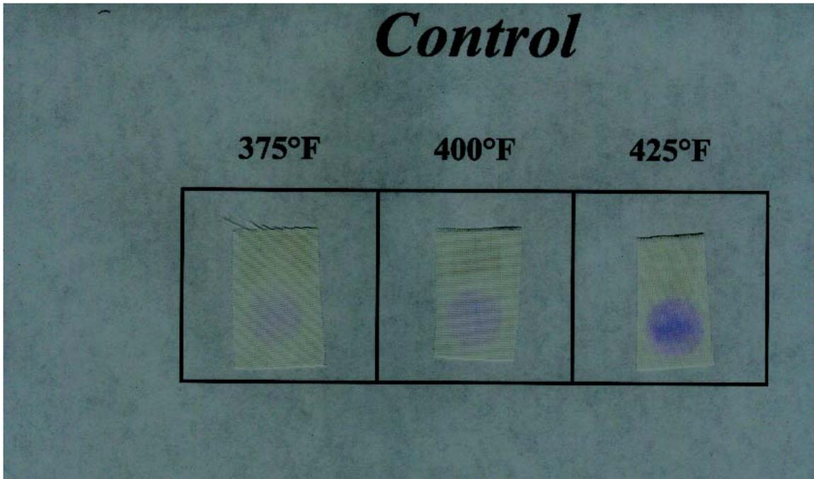
Figure 35. C.I. Disperse Blue 27 Vaporization in Control Samples.
