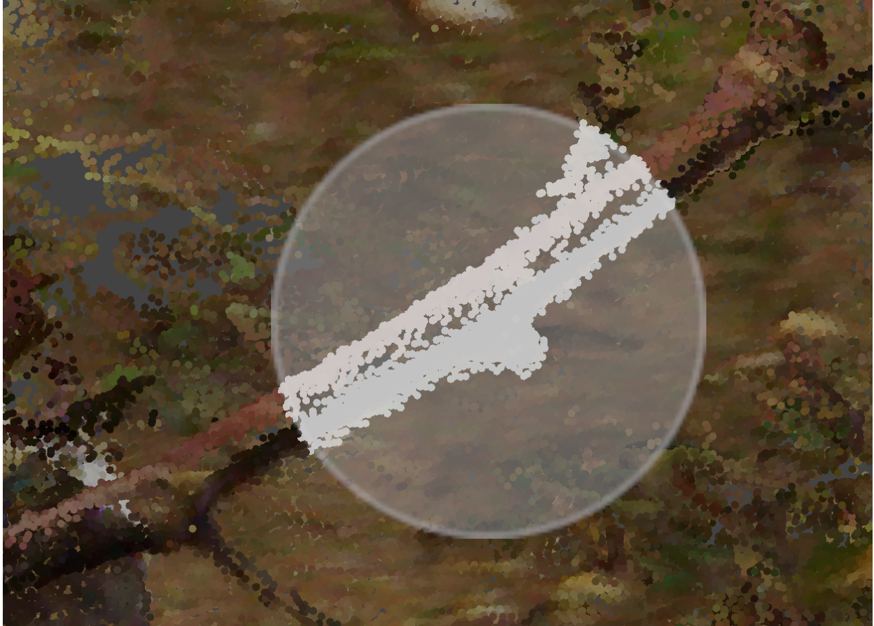
Figure 3.6: The highlight effect previewing the points that will be selected by a potential paint operation in the 2D interface. In this image, the depth limit feature is preventing the background points from being selected. The VR condition also has this highlight effect for points within the hand spheres.
