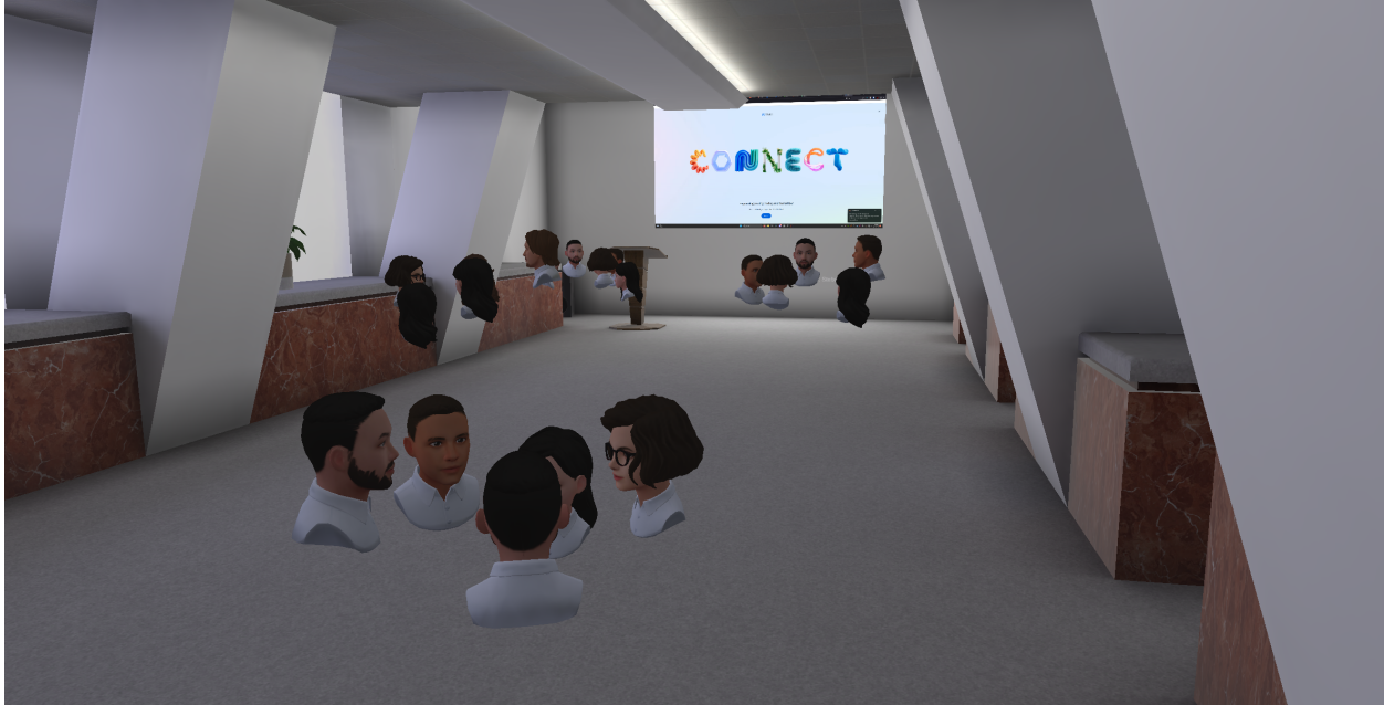
Figure 6.2: A versatile meeting space in conVRged . Due to spatial audio, users can talk in small groups without interrupting other conversations.
