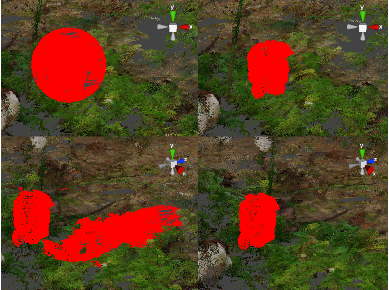
Figure 3.5: An example of the depth limiting algorithm used in the 2D system. The top images show the initial painted view. The bottom two images show the same cotton ball from a rotated perspective after the paint operation. The left two images have the depth limit turned off, and the right two have the feature turned on.
