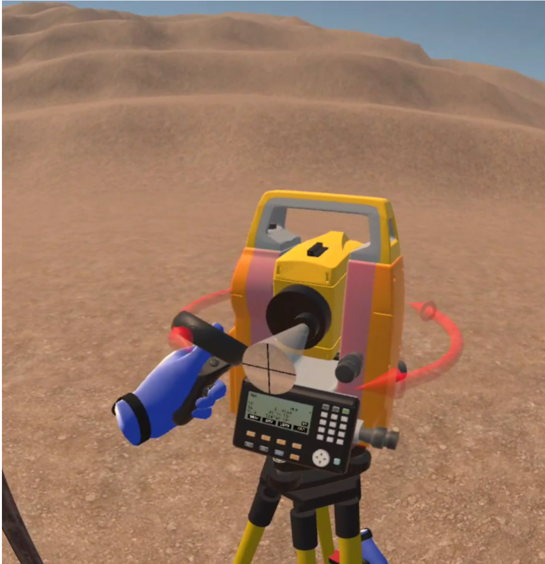
Figure 2.6: Course rotation of the station.
