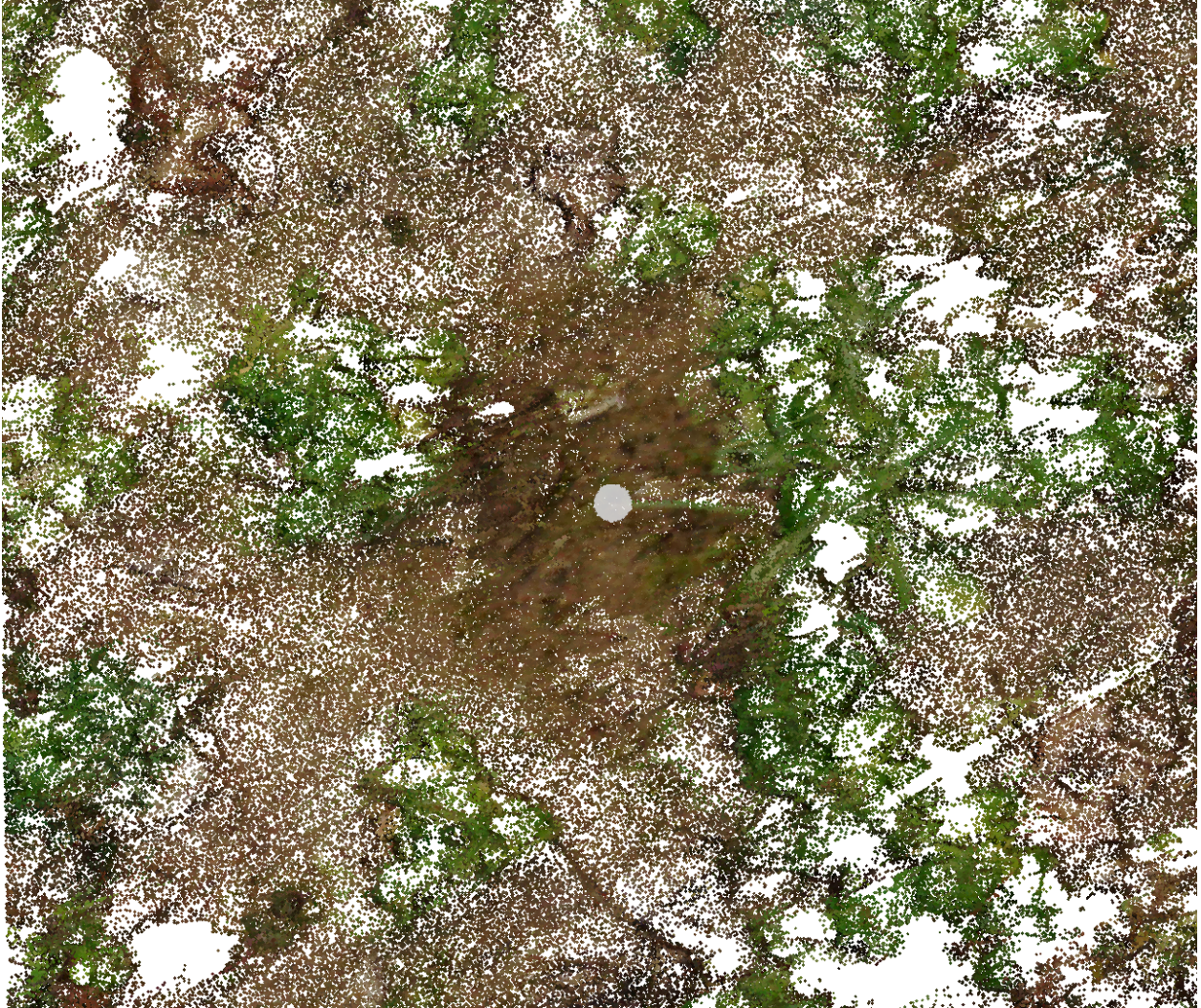
Figure 3.2: An example of the continuous LOD system used to render the point clouds. This system ensures that the full detail present in the source data is always visible in the area near the cursor/tracked hands, which happens to be in the center of the image here. The points in this image are reduced in size to exaggerate the low density areas and emphasize the effect.
