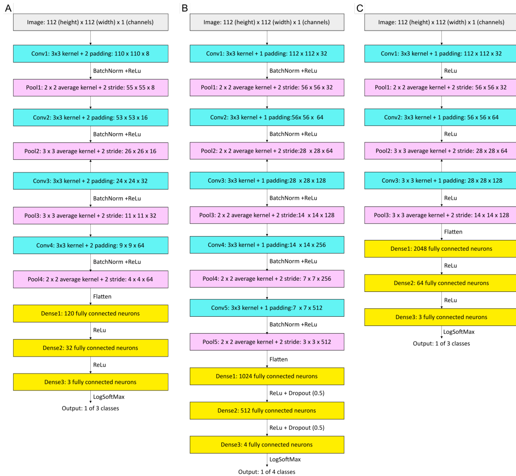
Figure 4.5: CNN model architectures for trait classification. A) Architecture for main stem promi-nence classification. B) Architecture for growth habit classification. C) Optimal architecture for TSWV infection level classification.
