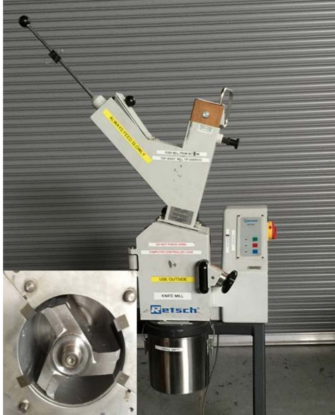
Figure 3.1. A laboratory heavy-duty shear cutting mill (Retsch SM 2000, Germany).
