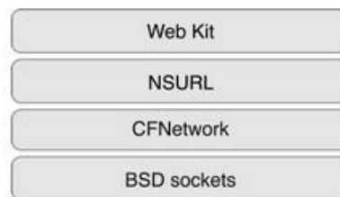
Fig. 2.3: The CFNetwork and software layers
