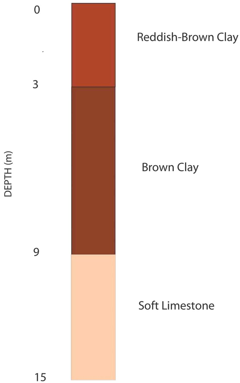
Figure 1.4: Borehole log for Well #44 obtained from the USGS Water Science Center in Atlanta, Georgia.
