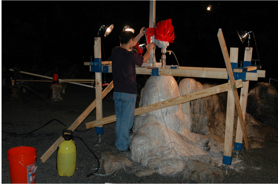
Figure 2.3. Platform built for drilling stalagmites at DeSoto Caverns (photograph by George A. Brook).
