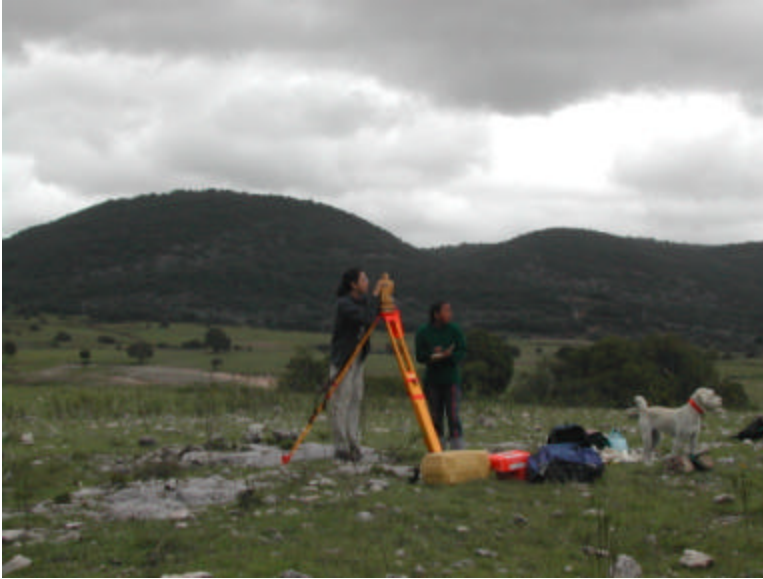
Figure 3.6 Mapping with total station on the hilltop of Nicayuhu .
