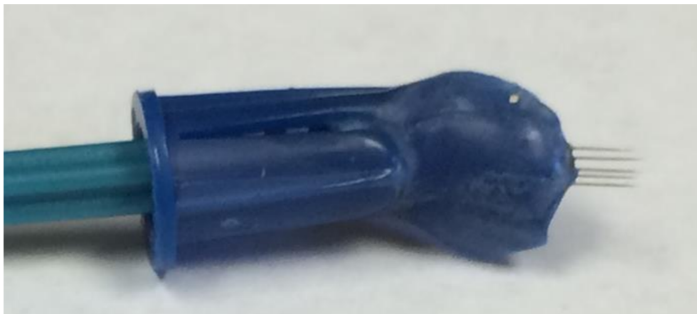
Figure 3.1. Inoculation fork used for inoculation of cucurbit seedlings with S. marcescens . The fork consists of a plastic bacterial loop handle attached to a melted plastic pen cap embedded with five fine-gauge needles.
