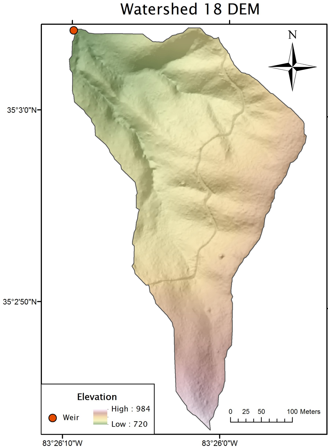
Figure 3.2: One meter resolution digital elevation model interpolated from bare earth LiDAR points on Watershed 18 of Coweeta Hydrologic Laboratory.
