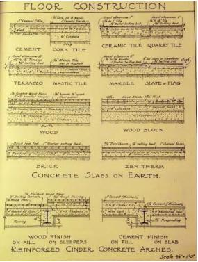
**Figure 17:** Floor Construction (1932 Ramsey, 79)
