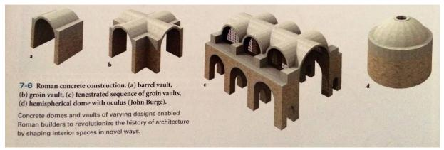
Figure 3: Roman Concrete Construction Diagram Showing the use of a Barrel Vault, Groin Vault, and Dome, Gardner's Art Through the Ages (Kleiner, p. 161)
