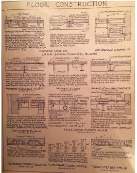
Figure 27: Floor Construction (1951 Ramsey, 79)
