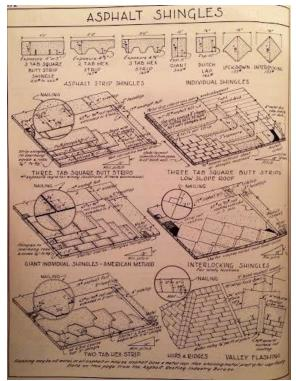
**Figure 34:** Asphalt Shingles (1956 Ramsey, 172)
