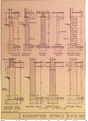
Figure 10: Foundation Details (Rouillion, 21)
