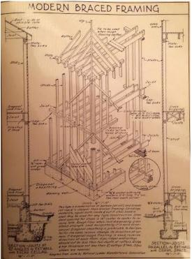
**Figure 21:** Modern Braced Framing (1951 Ramsey, 201)
