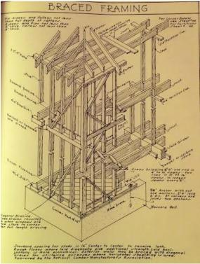
**Figure 11:** Braced Framing (1932 Ramsey, 93)
