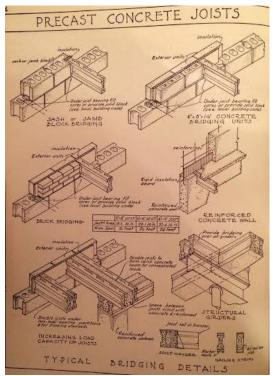
**Figure 26:** Precast Concrete Joists (1951 Ramsey, 74)
