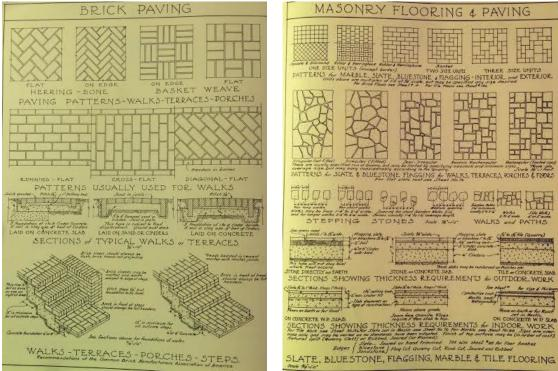
Figure 8: Masonry Flooring & Paving (1932 Ramsey, 5)
