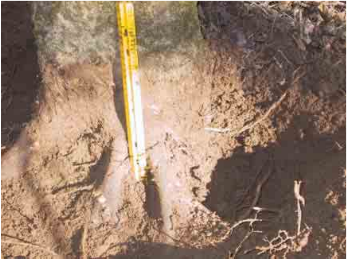
Figure 3.23 Example of an excavated tree within the Murder Creek watershed. Trees that appeared to have sediment accumulation around their tree boles were excavated and cored. Depths from the sediment accumulation around the tree bole to the top of the root crown were measured and recorded.
