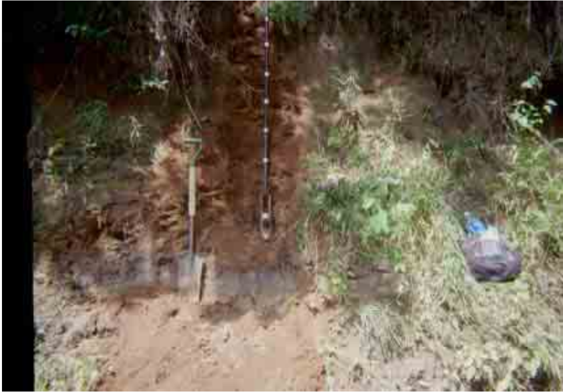
Figure 3.25 Picture of the Pre Historical Floodplain (PHFP) underlying the modern accumulation of the Historical Floodplain (HFP). The gray area represents reduced clay where the contact layer is high in clay content and there is little to no mica present in this horizon.
