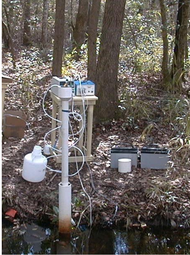
Figure 15. Photograph of Well 274 during an injection. Tracer was pumped from a carboy into the lowest (green) screened interval. A second pump was attached to the middle (yellow) screened interval, so that the upward movement of tracer could be monitored.
