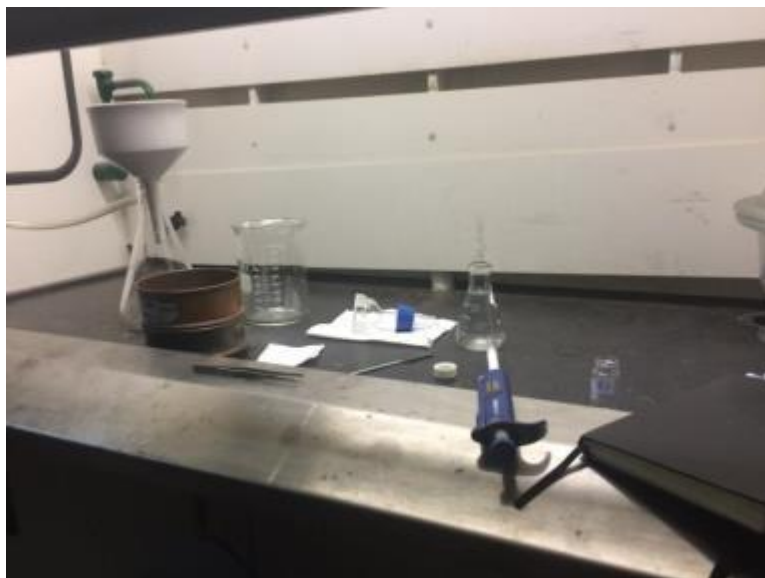
Figure 1: Testing area under clean fume hood used to sieve and filter nurdles from experiment 1: UV & thermal stress
