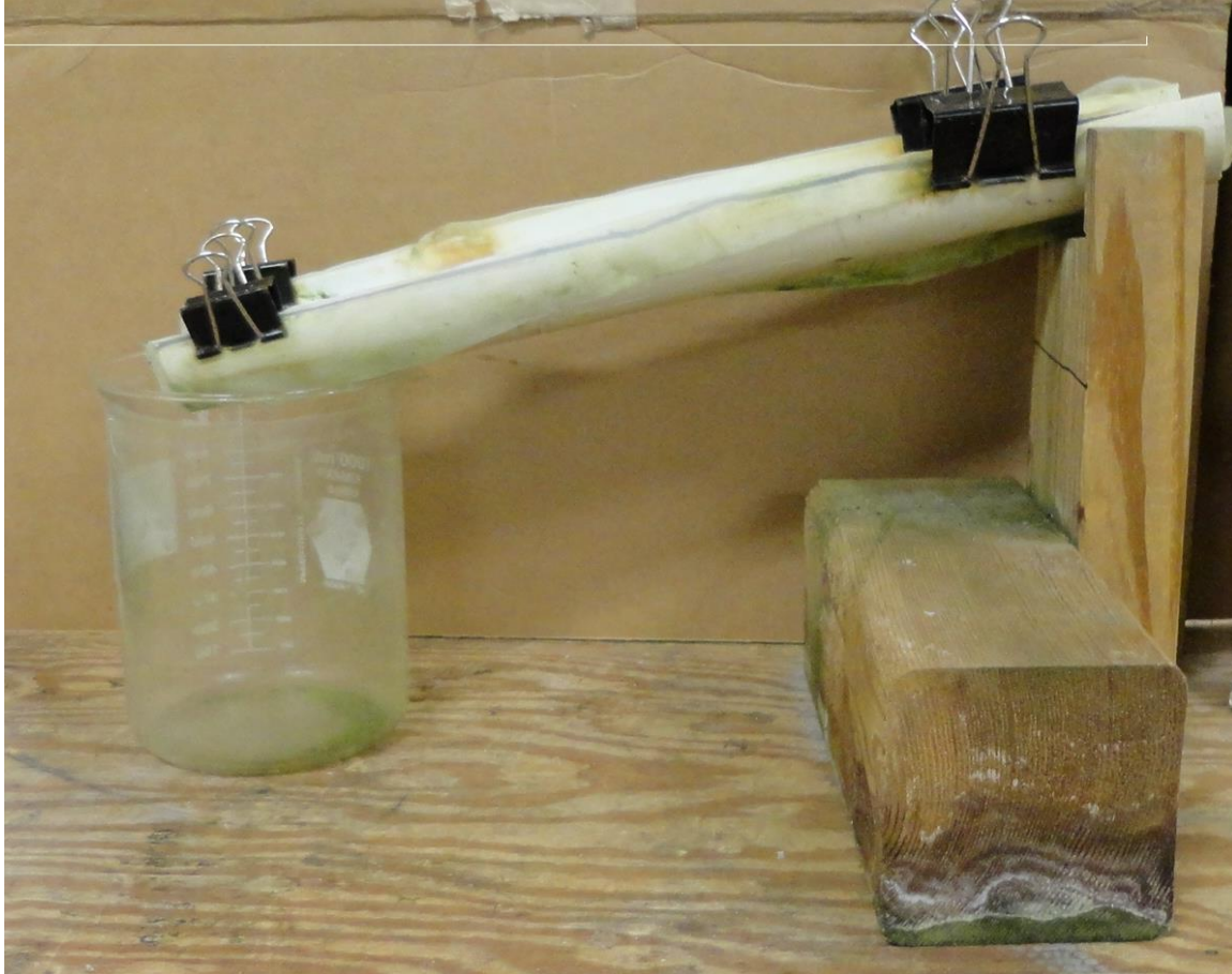
Figure 3.1: Biodeposit harvesting apparatus.
