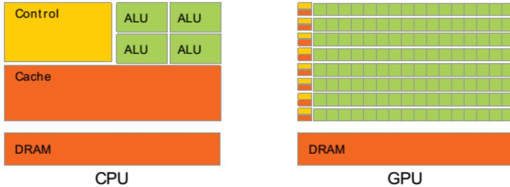
Figure 4: CPU and GPU architecture (Adapted version source: NVIDIA CUDA Programming Guide Version 5.5)
