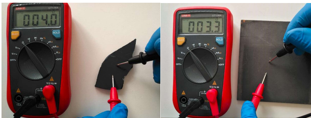
Figure S4.4. The electrical resistance of \text{Ti}_4\text{O}_7 ceramic electrode (Left) and graphite plate (Right) measured by multimeter.
