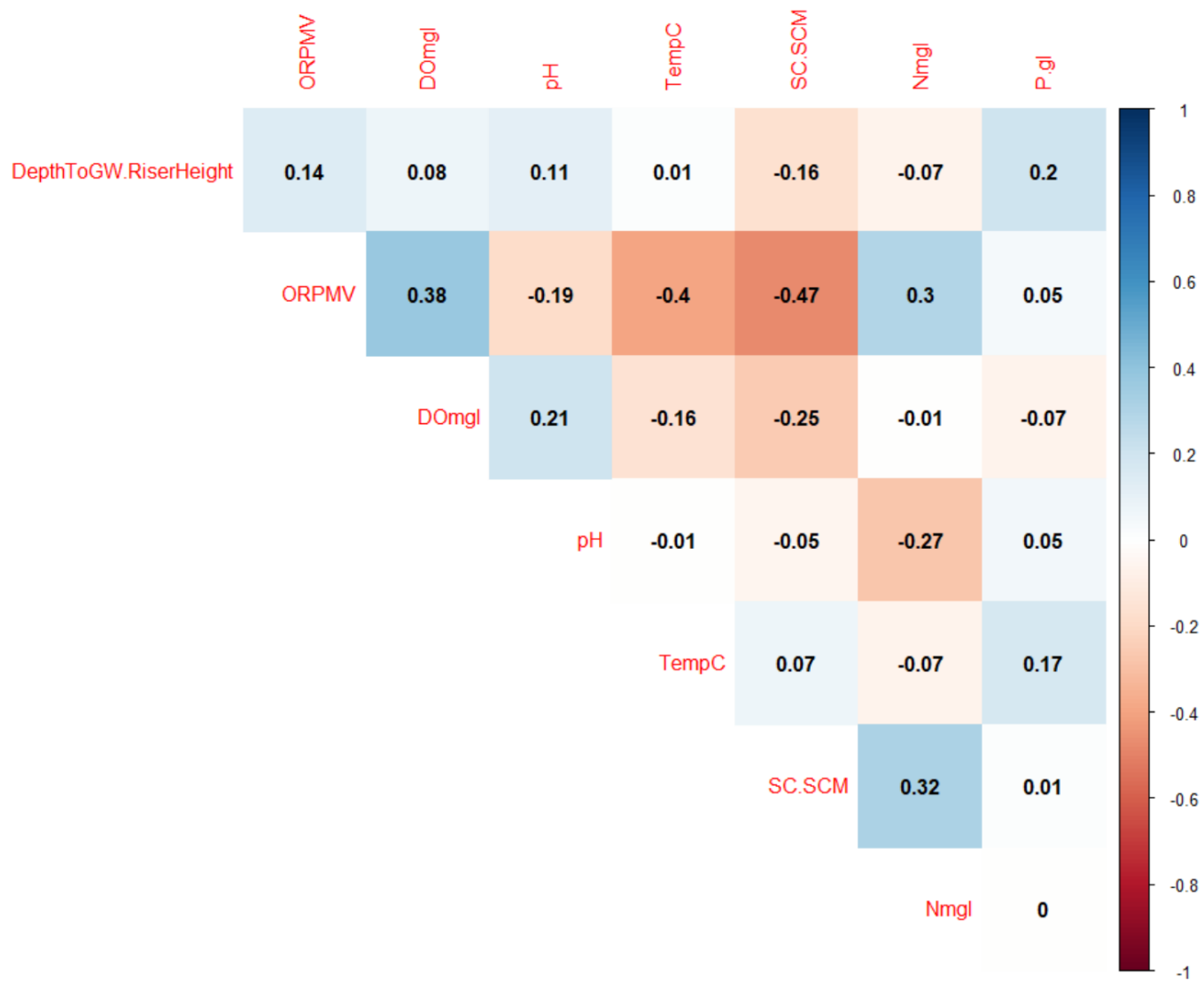
Figure 3.9: Correlation matrix of water quality and nutrients, no strong correlations exist but specific conductivity and ORP are moderate positively related to nitrate + nitrite.
