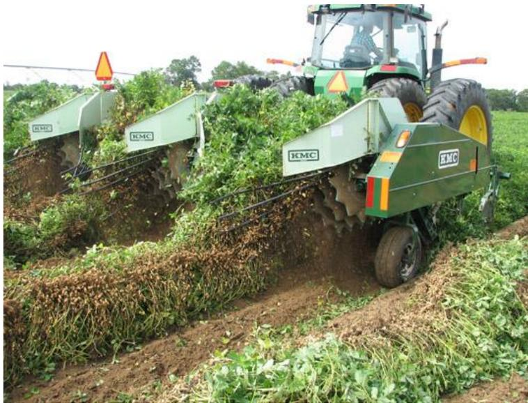
**Figure 1.1: Peanut digger inverting peanuts for drying in windrows**
