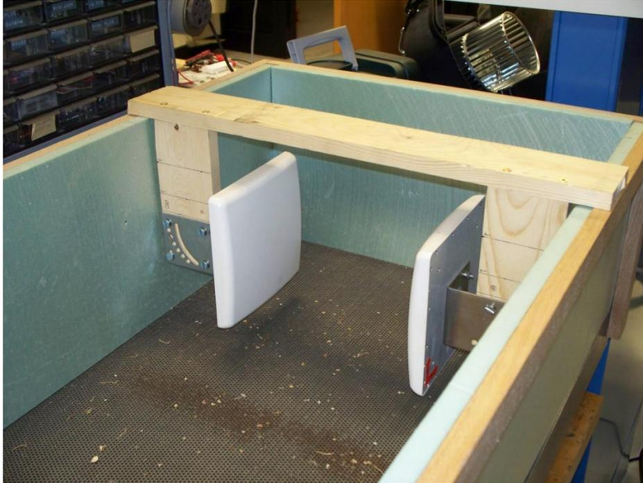
**Figure 11.11: Antennas mounted within drying trailer**
