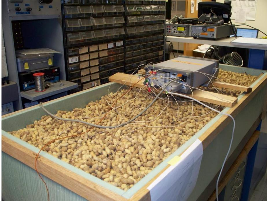
**Figure 11.10: Drying trailer shown with thermocouples placed throughout**
