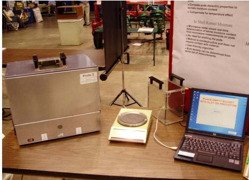
**Figure 10.1: Previous version of microwave moisture meter (controlled by external laptop)**
