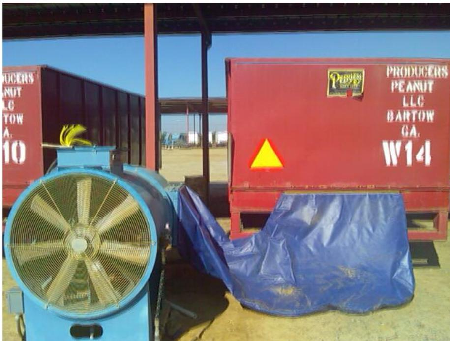
**Figure 4.3: Peanut drying trailer connected to BlueLine dryer**
