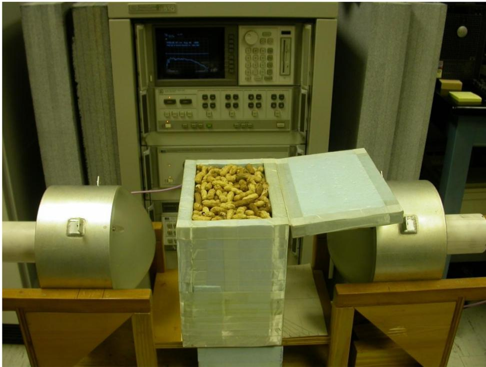
**Figure 6.3: Free-space measurement system with vector network analyzer**
