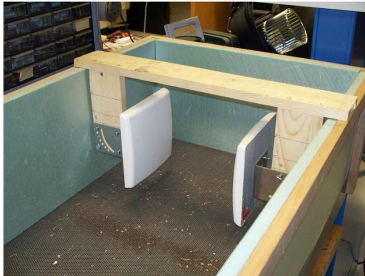
**Figure 8.3: Antennas for microwave meter mounted within drying trailer**
