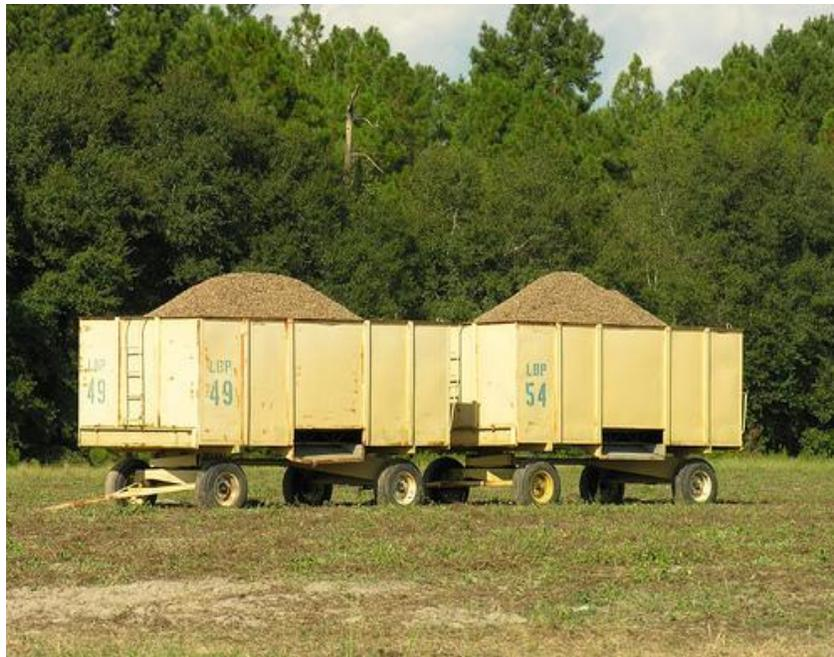
**Figure 4.1: Wagon-type peanut drying trailers loaded with peanuts**
