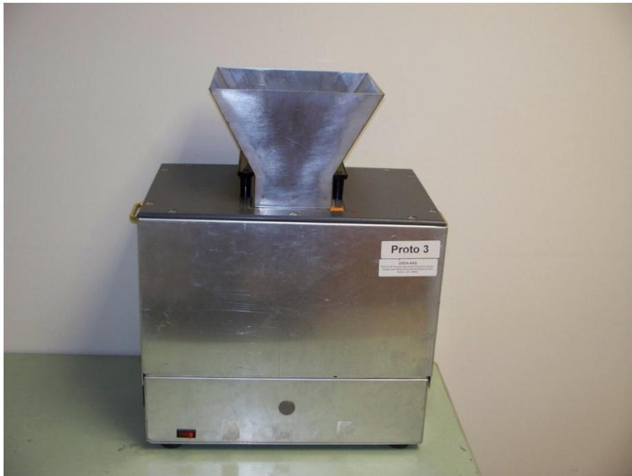
**Figure 6.5: Enclosed version of microwave moisture meter**
