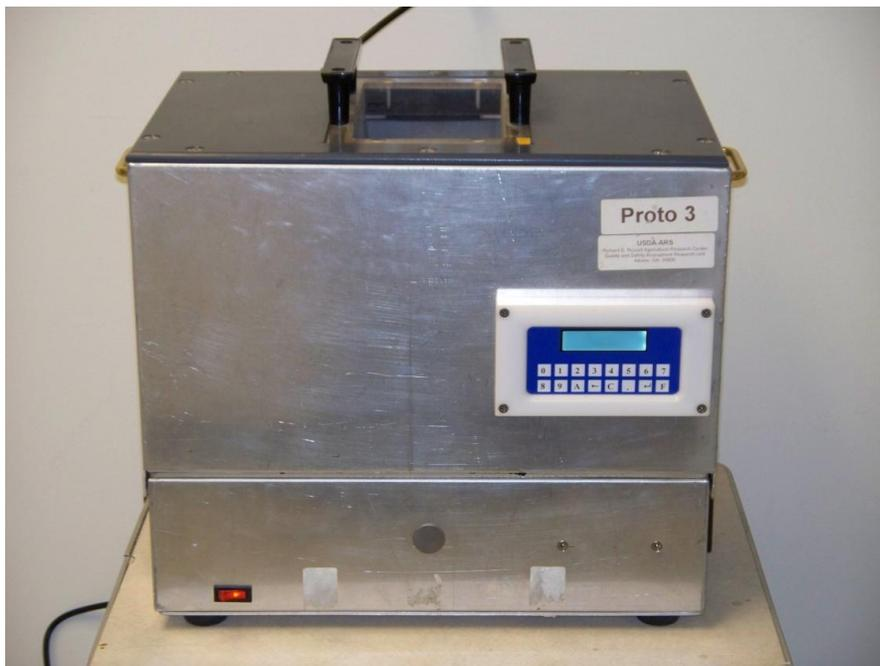
**Figure 10.9: Microwave moisture meter shown with LCD and keypad (embedded system)**
