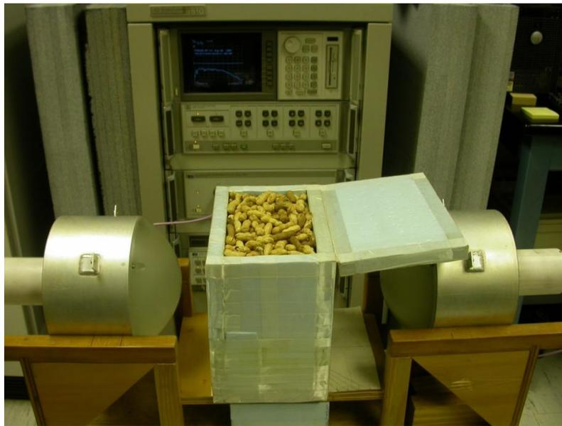
**Figure 9.1: Free-space measurement system with pod sample shown**
