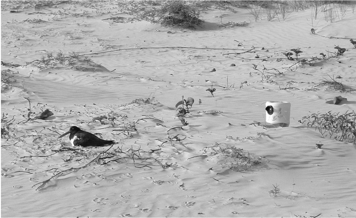
Figure 2.2. Each camera was mounted on a wooden stake, placed approximately 1.5–2 m from a nest, and protected by a cutout plastic bottle. An 18.3-m cable buried 2–3 cm in the sand substrate connected each camera to a recorder and battery
