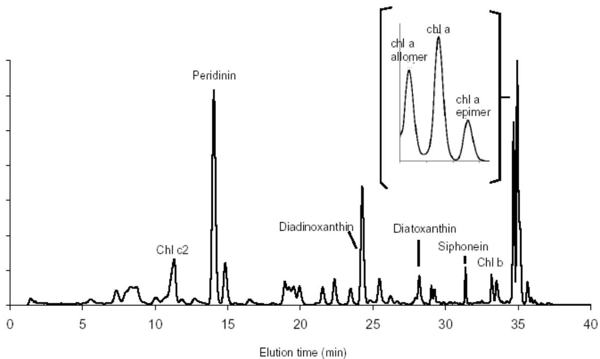
**Figure B.3** Typical C-8 elution profile monitored at 450 nm for methanol-soluble pigments extracted from whole coral fragments using the methodology of Zapata et al. (2000).
