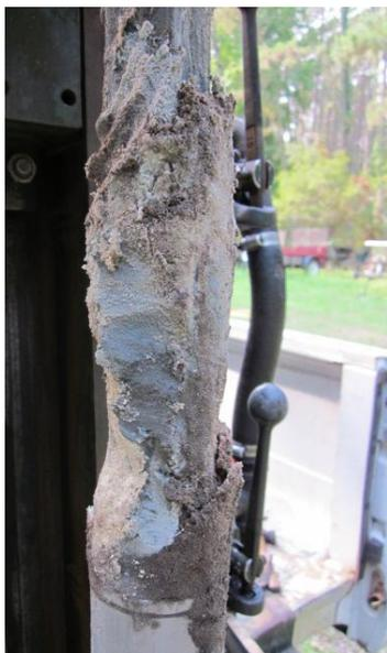
**Fig. 4.12** Clay atop the mandril (where top of core tube attaches to truck-mounted Giddings corer) in core UGA 0m
