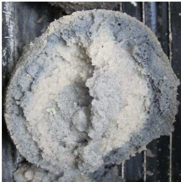
**Fig 4.13** Gleyed clay pushed out by compaction pressure to form artificial ring around sandy sediments in core UGA 50m
