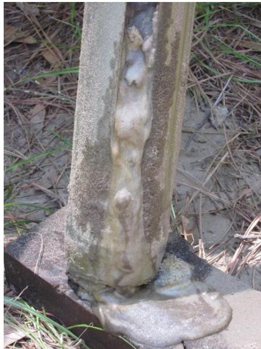
**Fig. 4.14** Saturated sediment oozing from the open slit and base of the core tube in core GCF 50m
