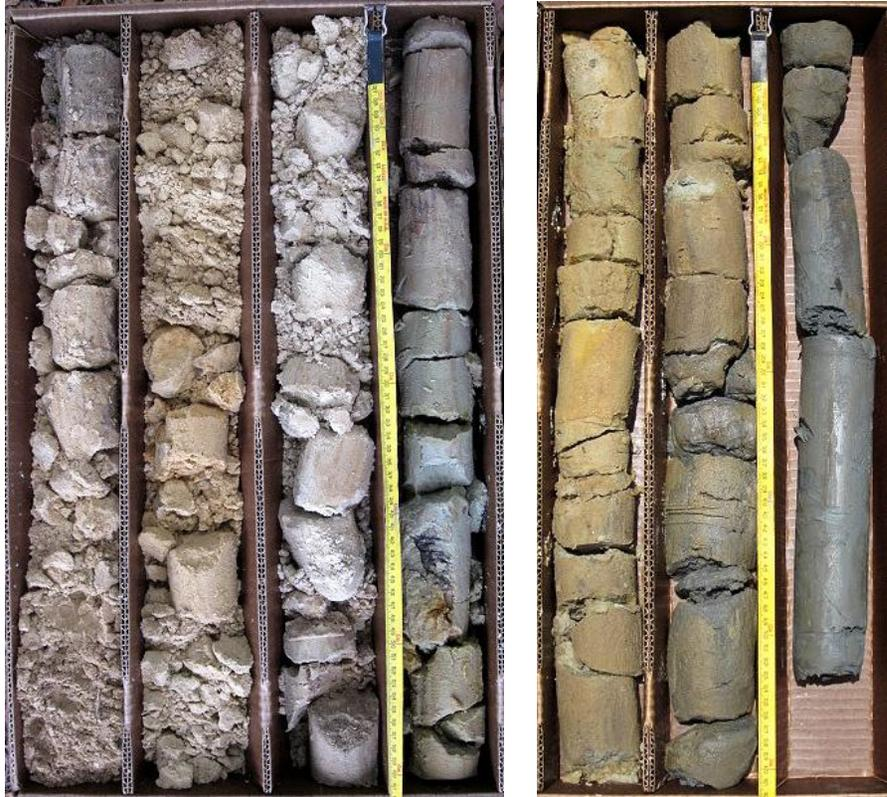
**Fig. 3.10** All B 0m cores stored in boxes after collection. Note the absence of a well developed A horizon. Scale: Each column is 62 cm long. Core lithology, contents, and Munsell colors are represented in the diagram.
