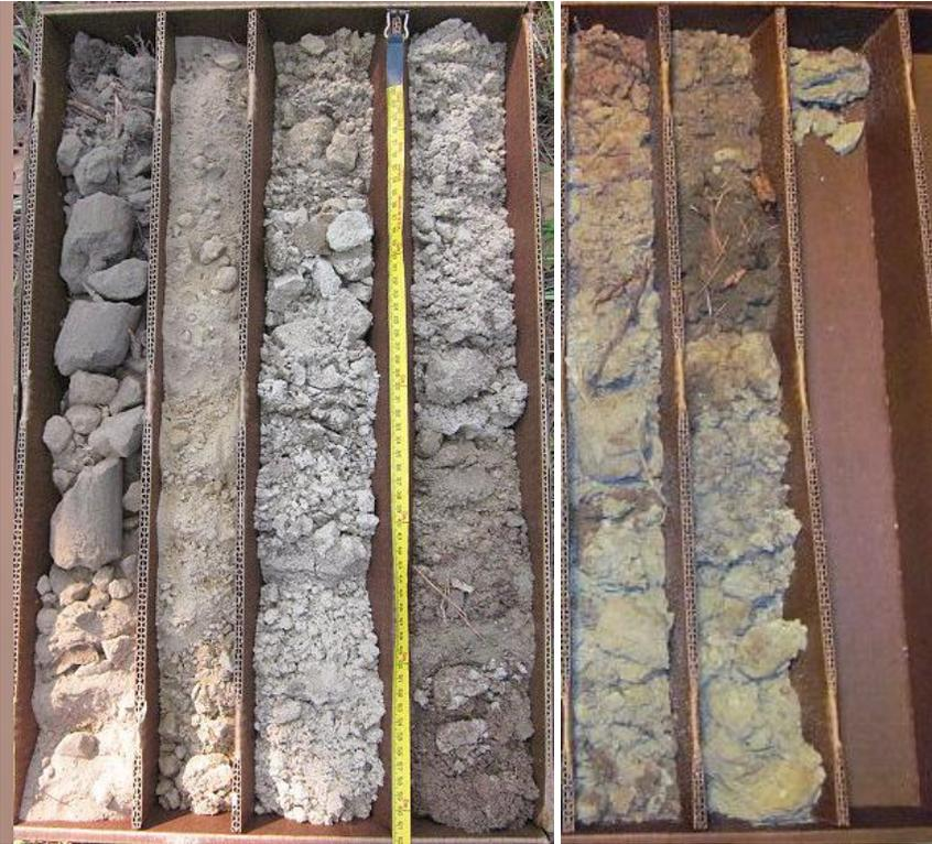
**Fig. 3.18** All GCF 100m cores stored in boxes after collection. Note the contaminated areas towards the bottom of the fourth column and top of the sixth column where pine straw and leaf litter from the surface are evident; these areas of contamination, a total of 20 cm, were subtracted from the total core length, and are not included in the diagram to the right. Scale: Each column is 62 cm long. Core lithology, contents, and Munsell colors are represented in the diagram.
