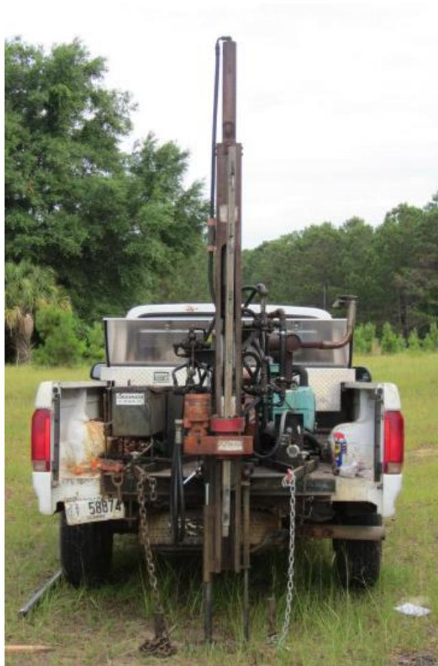
**Fig. 2.1** The truck-mounted Giddings hydraulic soil coring system used to collect sediment cores.
