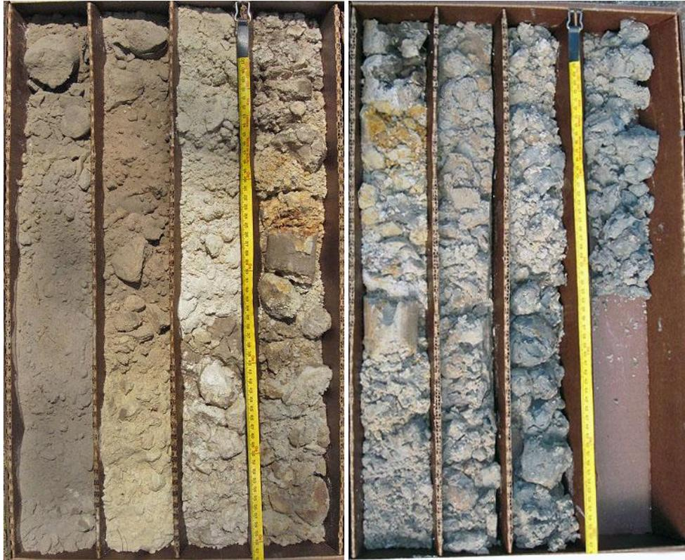
**Fig. 3.17** All GCF 50m cores stored in boxes after collection. Scale: Each column is 62 cm long. Core lithology, contents, and Munsell colors are represented in the diagram. Note the increase in silt and clay just above 200 cm; this sedimentologic change represents accumulation of finer grained particles around fine roots.
