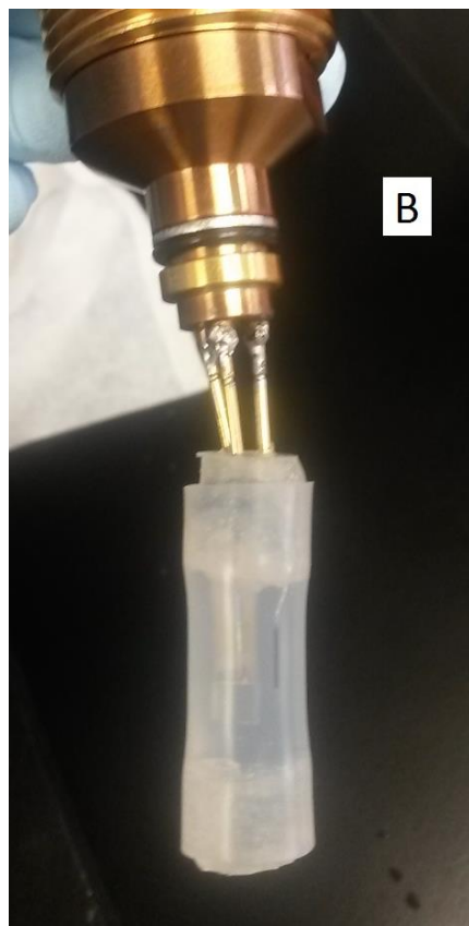
Figure 3.11. Finished prototype. (a) electrode cap (b) completed cell design attached to electrochemical cell lid
