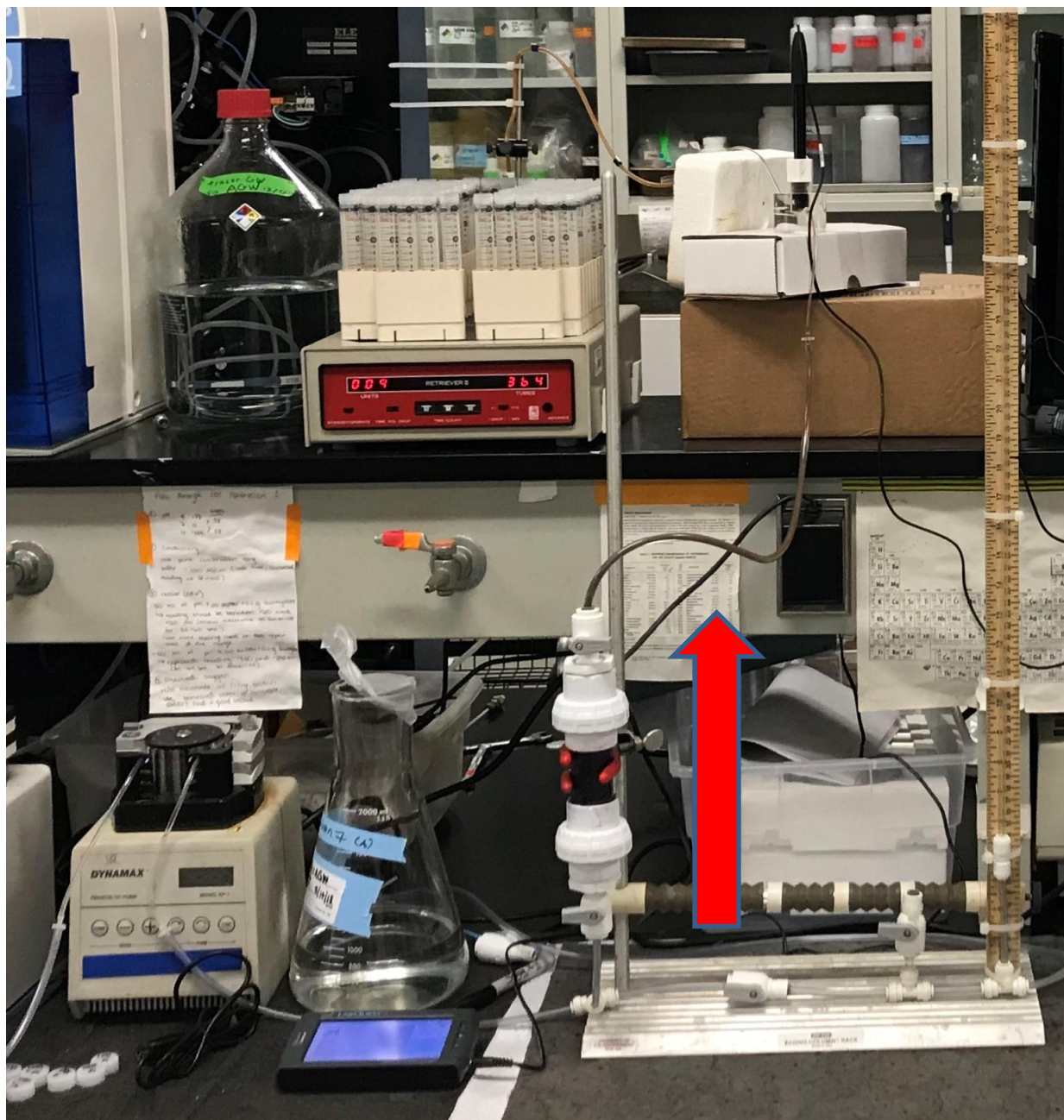
Figure 3.1: Image of the experimental column system with flow in an upward direction
