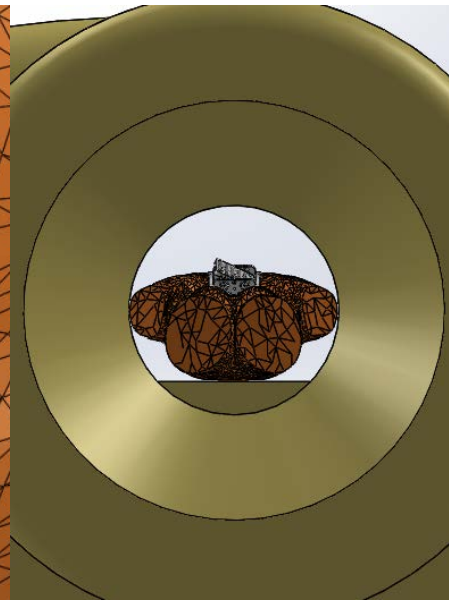
Figure 4.2 - (a) The positioning device, including template and support structure. (b) Top view of template, showing full grid of holes and the five wells with fiducial markers. (c) CAD image demonstrating the positioning of SpinoTemplate above the lumbar spinal cord. (d) Substantial clearance within a 60cm closed-bore scanner.
