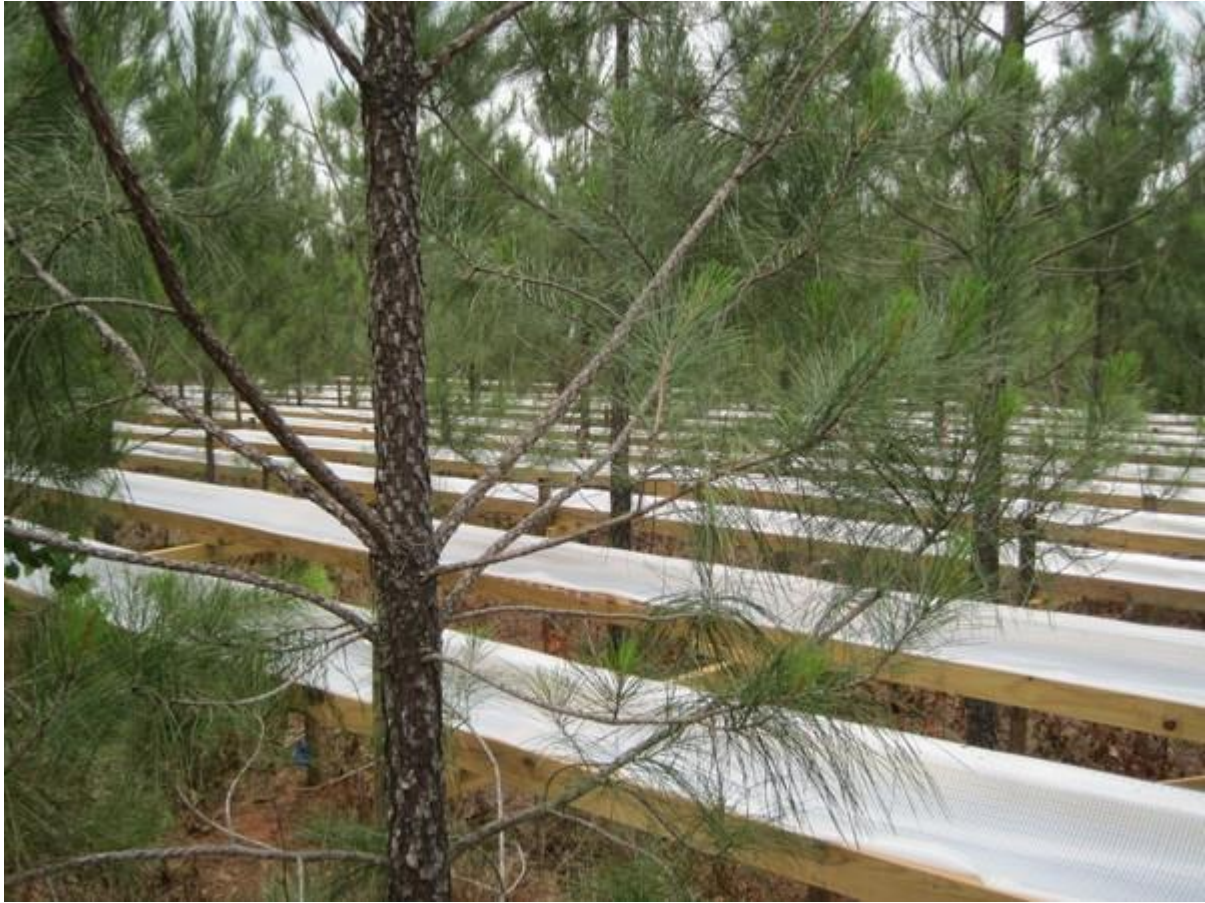
Figure 3.1. Throughfall reduction structure covering ~30% of the plot area with troughs to capture and funnel throughfall away from the plots. Taliaferro County, Georgia in 2012 when trees were 6 years old.
