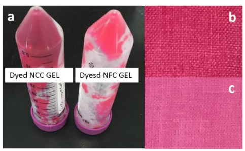
Fig. 3.4. Dyed enzyme-treated NFC and NCC (a) dyed cotton fabric with enzyme-treated NFC (b), and dyed cotton fabric with enzyme-treated NCC (c)
