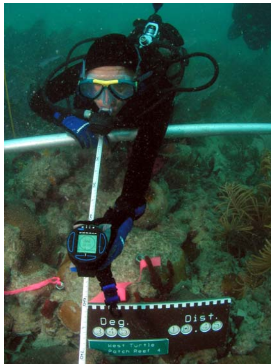
Figure 6. Photograph of the author checking the position of a diseased coral colony during the diseased coral survey. The diver is positioned at the station's stake, aiming the digital compass in the direction of the coral colony of interest.
