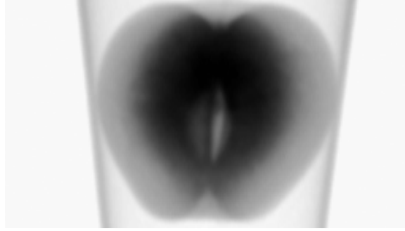
Figure 2.2: Scout scan of an apple secured to the specimen stage in a plastic drinking cup. Darker shades indicate higher x-ray absorption.
