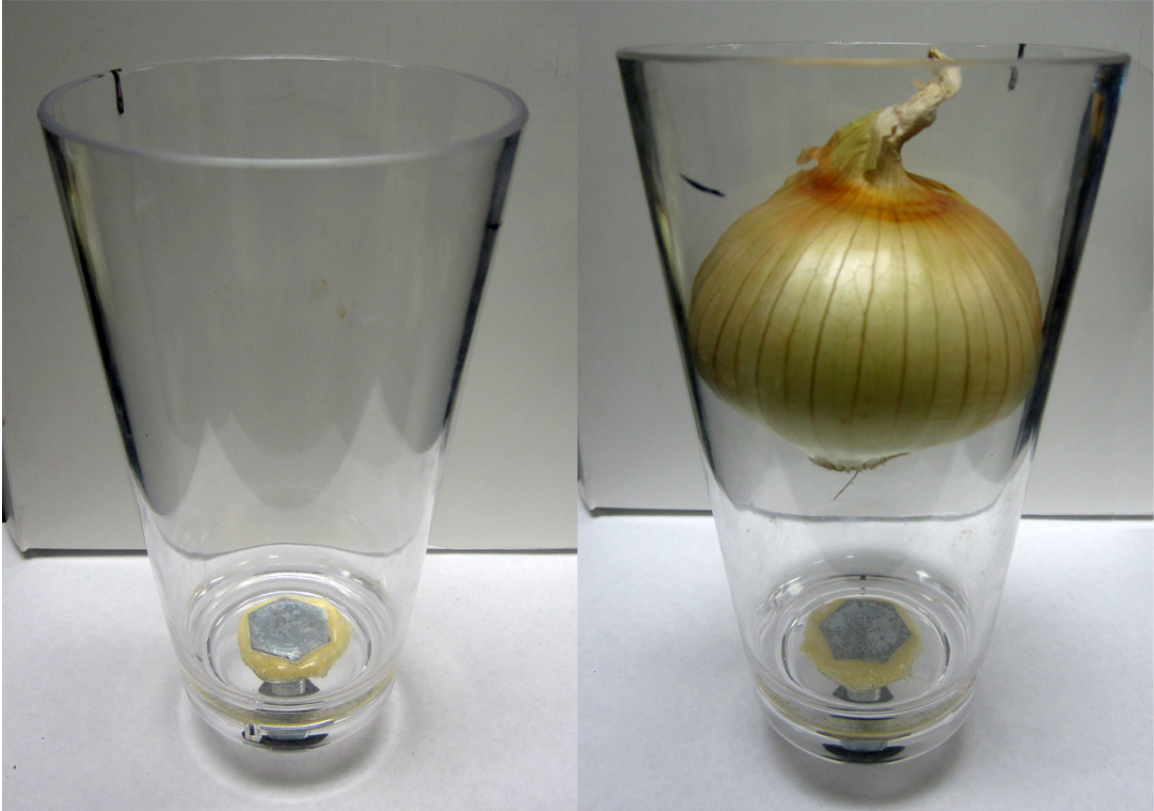
Figure 3.2: First onion holder built out of a plastic drinking cup.
