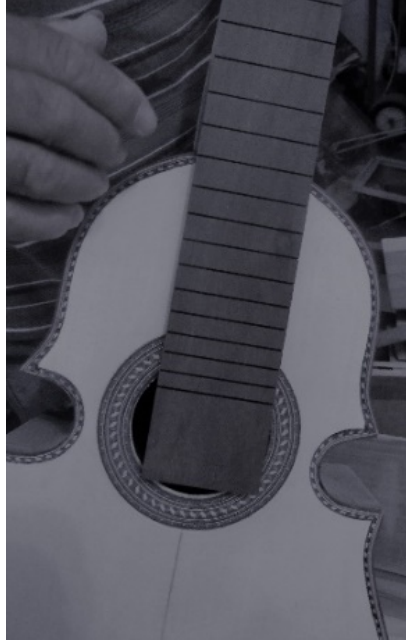
Figure 2.2: Cuatro Construction, Front (Without Strings)
