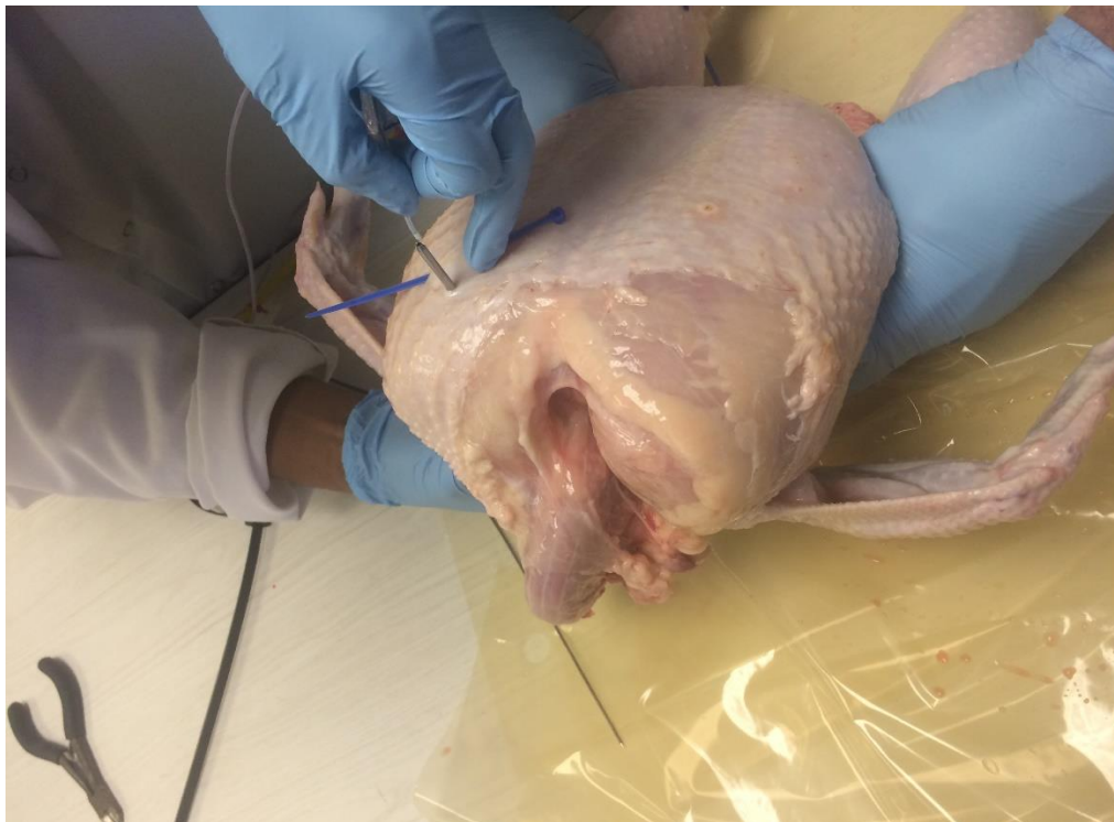
Figure 2. A multi-probe (5-probe) t-type thermocouple was inserted in the breast muscle of the chicken carcass.
