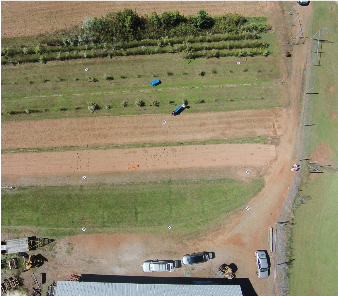
Figure 3.3: Aerial view of Test Site 2 containing ground control points and target of known volume in Whitehall Forest.
