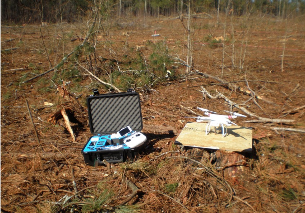
Figure 3.4: Unmanned Aerial System(UAS)(DJI Phantom 2 Vision Plus quadcopter)
