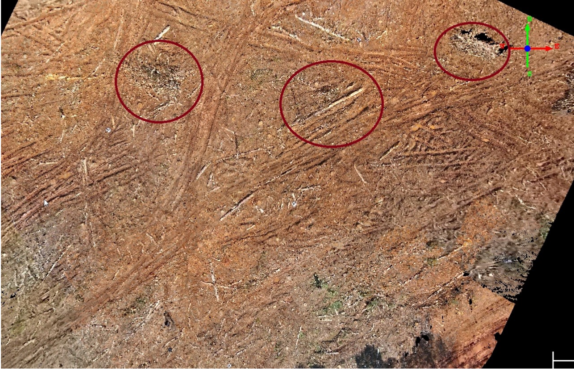
Figure 4.1: 3D image with residue piles identified. Volumes associated with these piles were not included in either mini plot or line intersect sampling. They appear to be responsible for differences in volume estimates between field sampling and 3D image sampling.
