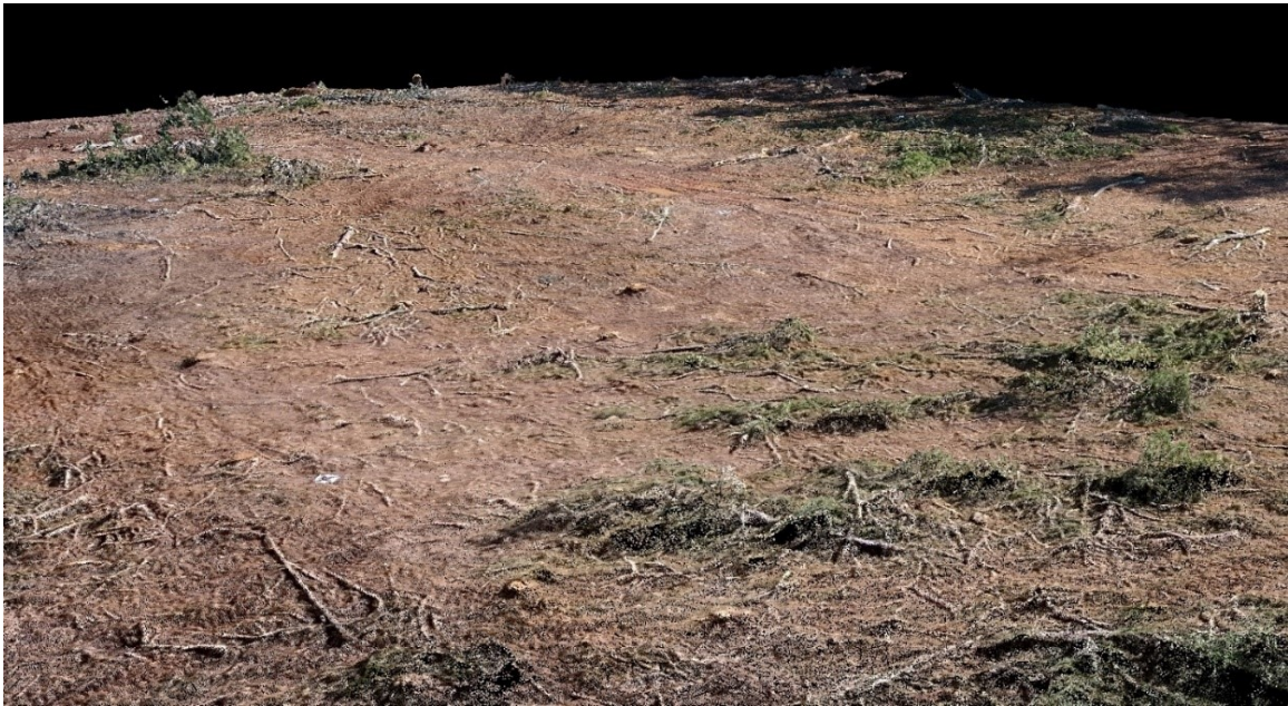
Figure 1.1: Test plot: Three-dimensional point cloud image of the woody residue remaining on a recently harvested forest site. This model is generated using the images extracted from the video taken by the small camera of the UAS and georeferenced using the five targets set up in the field.
