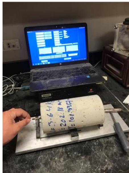
Figure 6-27: Dynamic Modulus of Elasticity Test Configuration
