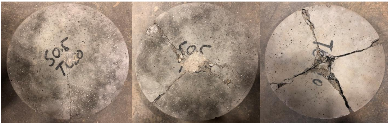
Figure 6-34: Progression of Cracks Measured in Drop Weight Hammer Test: (a) Initial Crack, (b) Control Failure, and (c) Complete Failure
