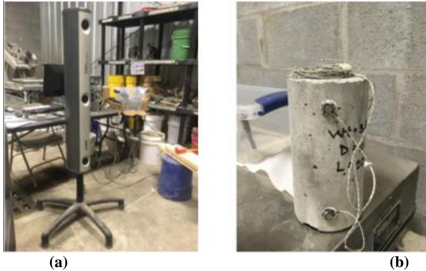
Figure 6-25: Static Modulus of Elasticity Test Configuration (a) Motion Capture Camera (b) Detection Sensors
