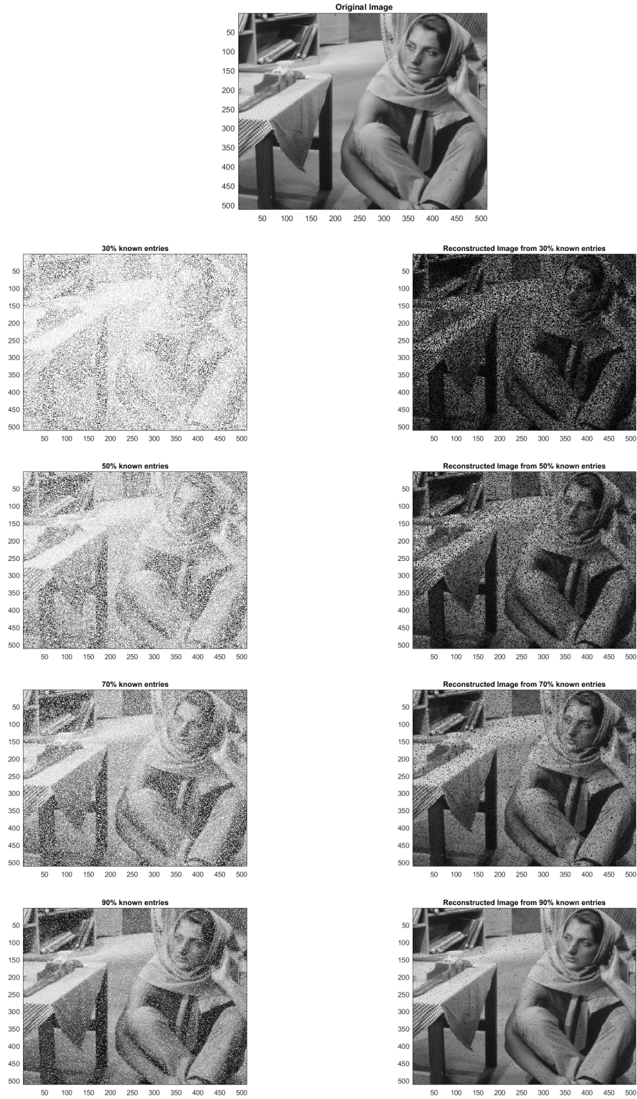
Figure 2.1: Top row: The original image; Rest of the rows: left column correspond to image with missing entries and right column images are reconstructed using APA described in section 2.3 from the corresponding images on left
