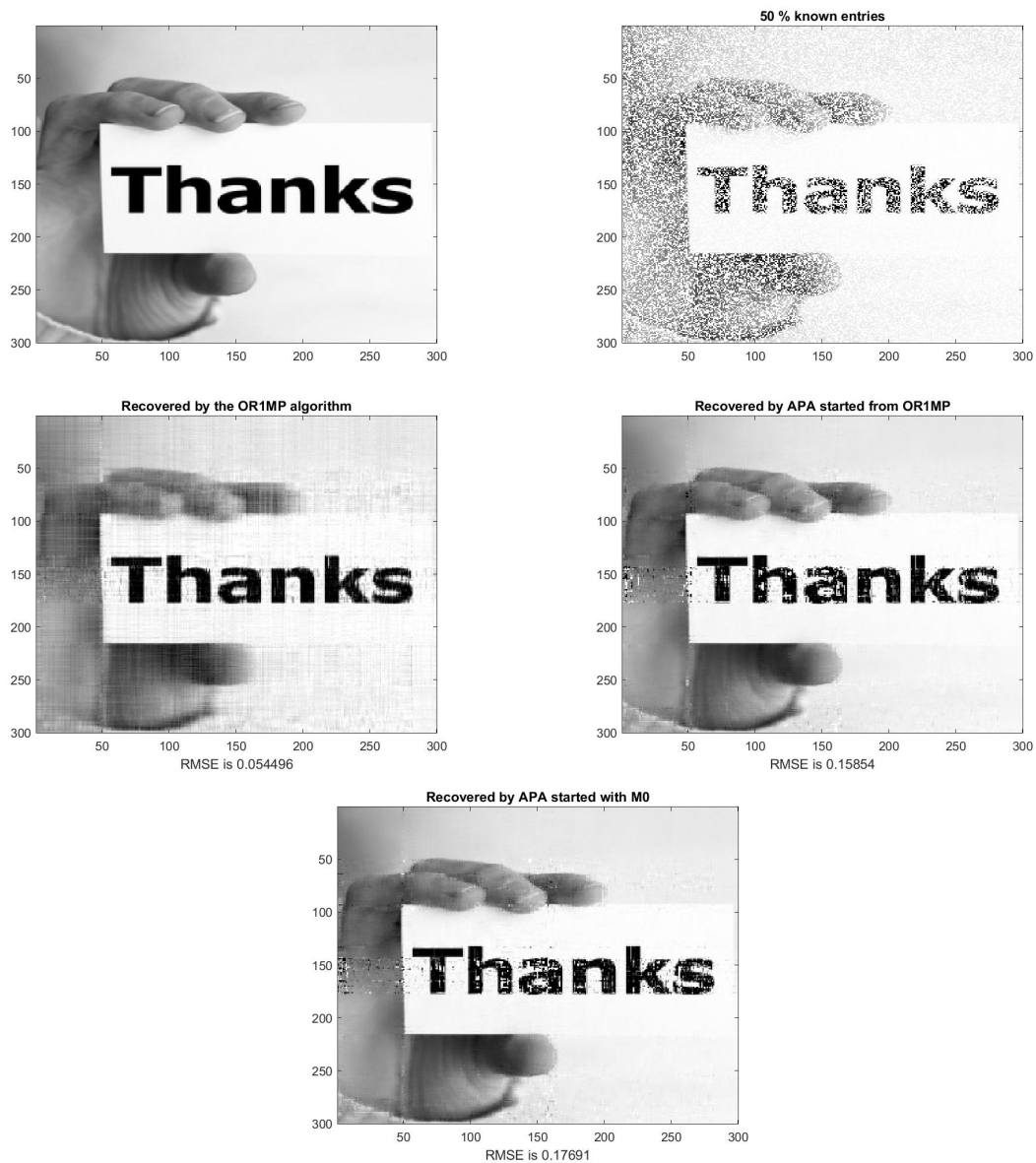
Figure 4.4: Top row: The original image and the image of 50% known entries; Rest of the rows: Outputs from Algorithm OR1MP, Algorithm 4 with initial guess from the Algorithm OR1MP and Algorithm 4 from the 50% known entries based on rank 25.
