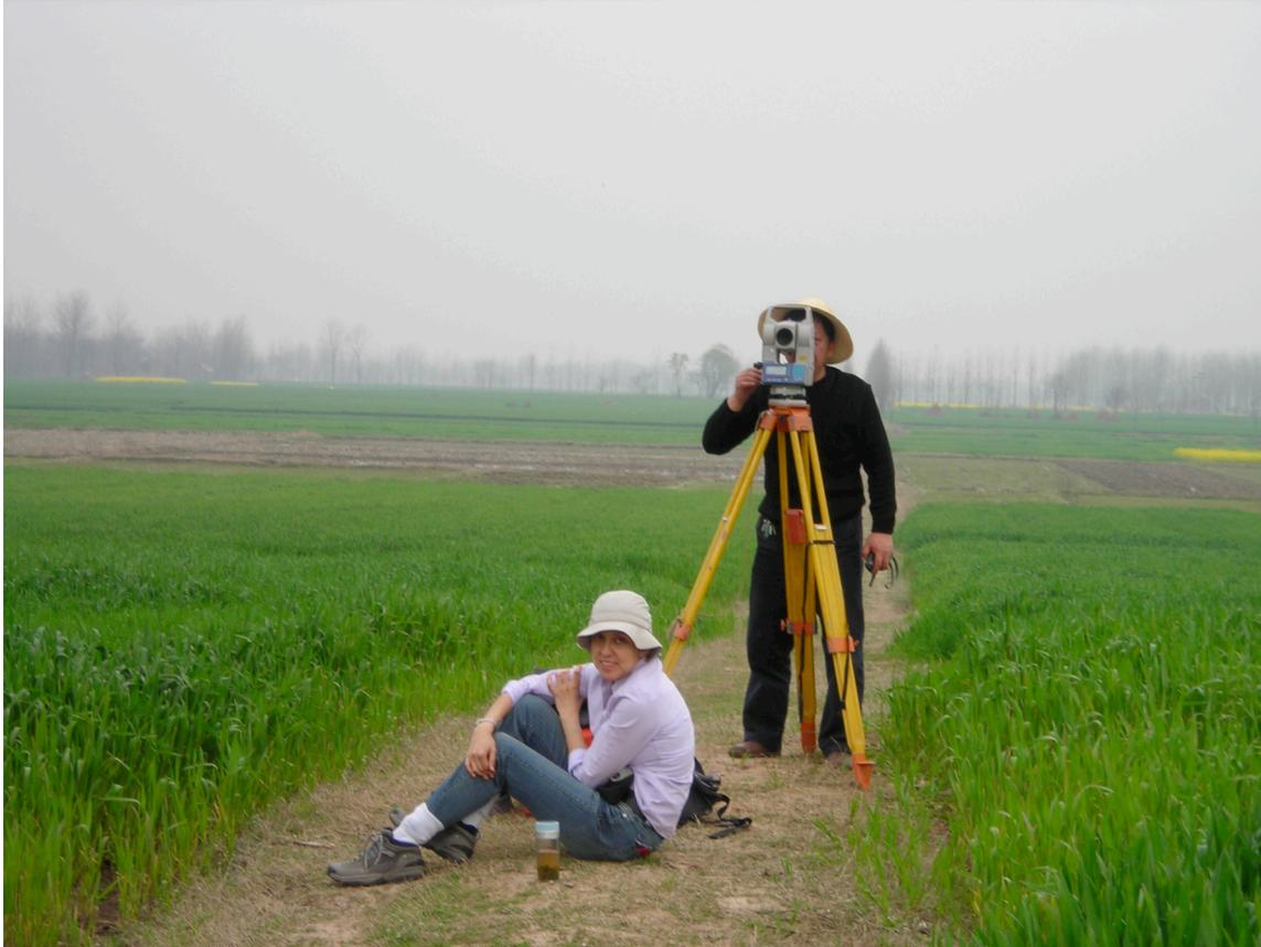
Figure 3.4 Mapping Huangtucheng using a total station.
