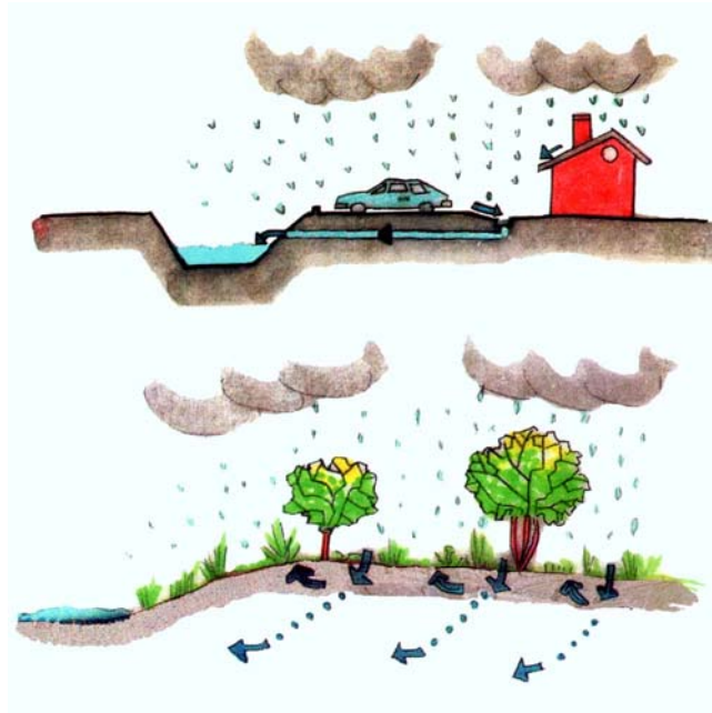
Figure 3.3 Jen Uncapher, Runoff is worse on impervious surfaces than vegetated soil.
