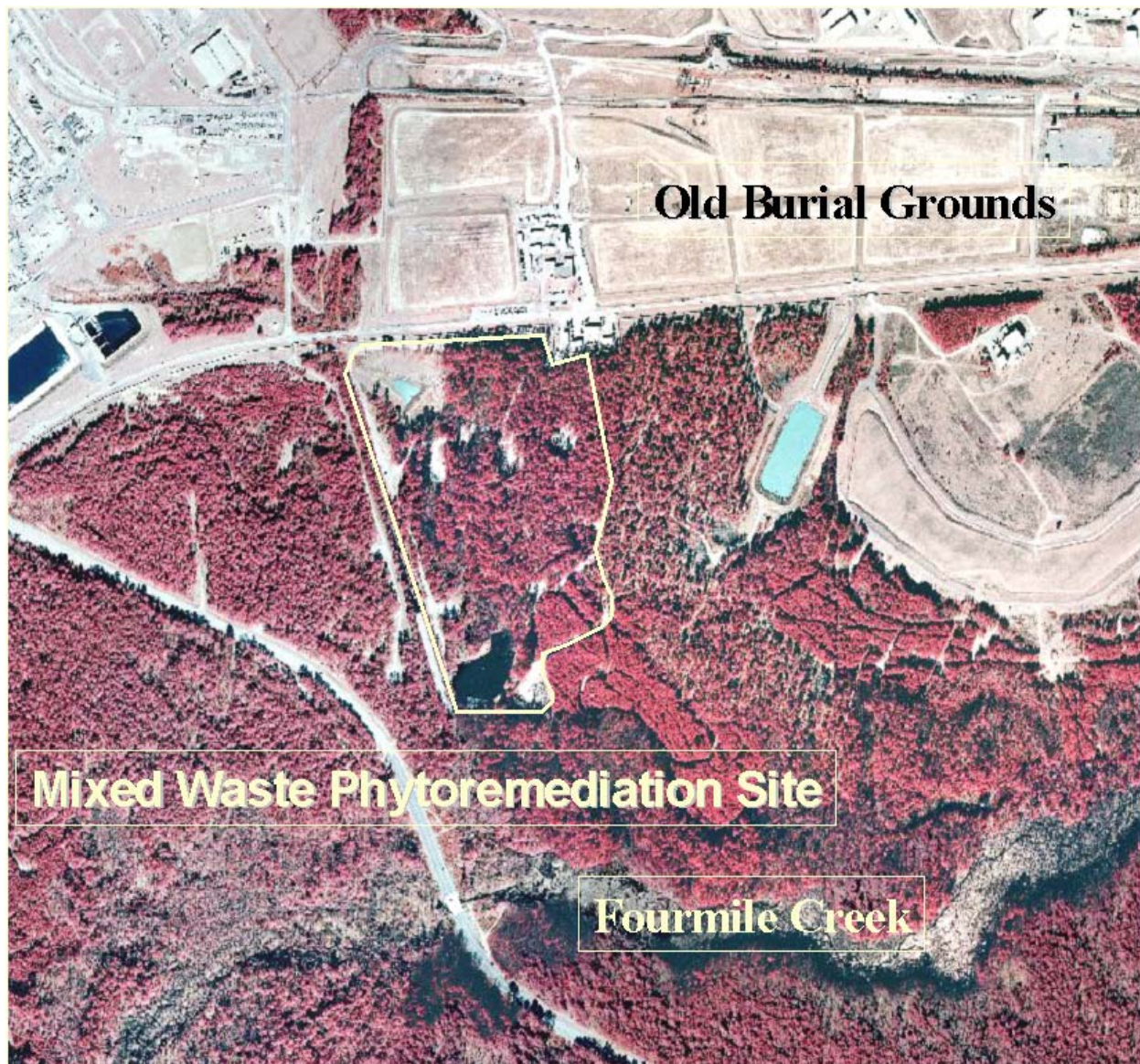
Figure 2-1 – The Mixed Waste Phytoremediation Site is utilizing a new disposal technique that consists of irrigating a hardwood/pine forest with tritiated water to reduce the concentration of tritium flowing from the Burial Grounds into Fourmile Creek.
