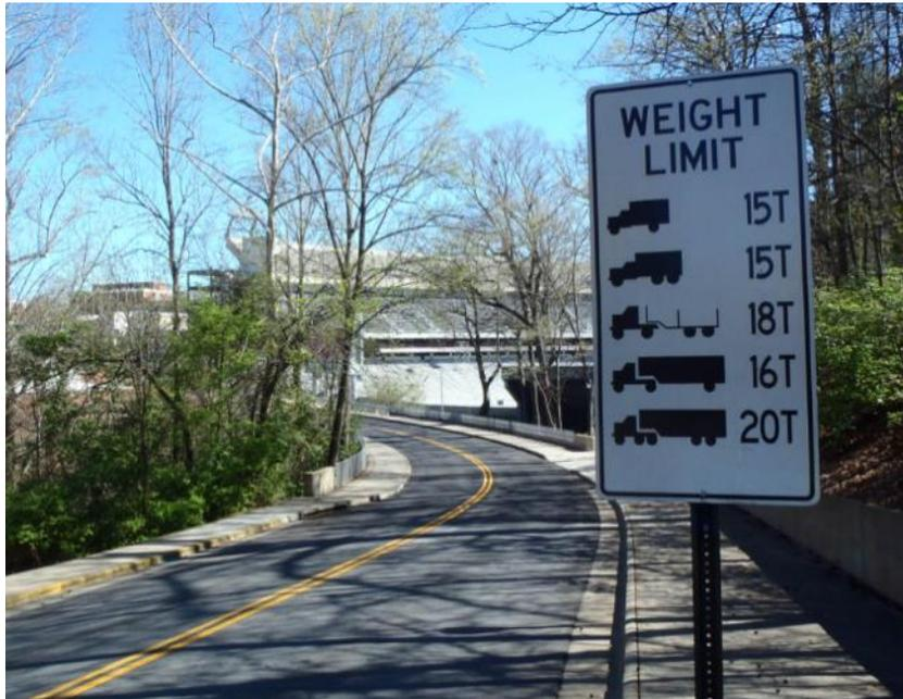
**Figure 9—Bridge Weight Limits [GDOT, 2017]**
