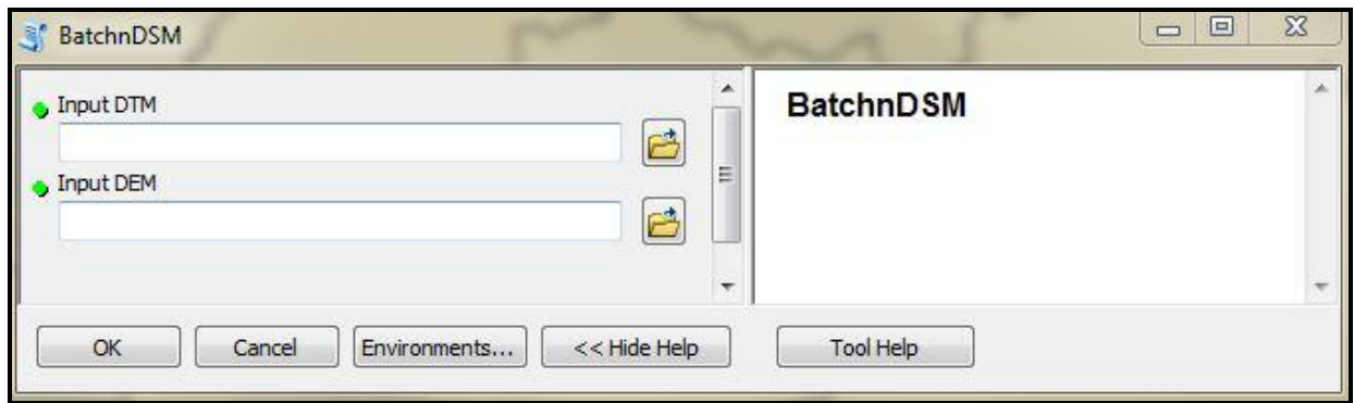
Figure 2.10 - BatchnDSM software tool created using a Python script to iteratively process raster files
