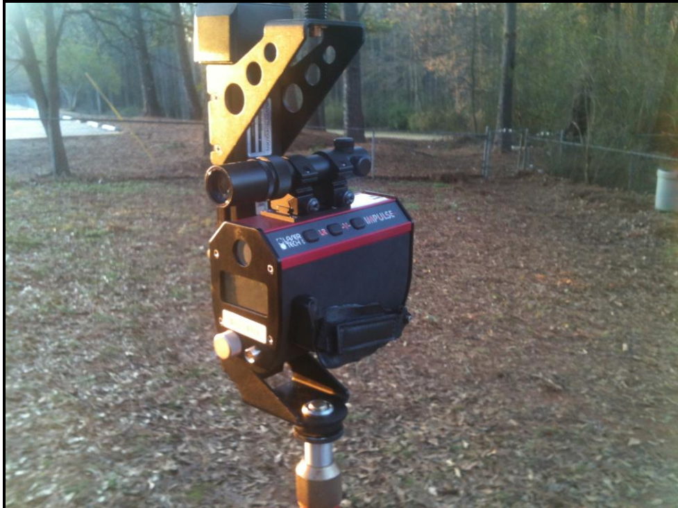
Figure 1.6 - Impulse 100 laser rangefinder with clinometer used in the study
