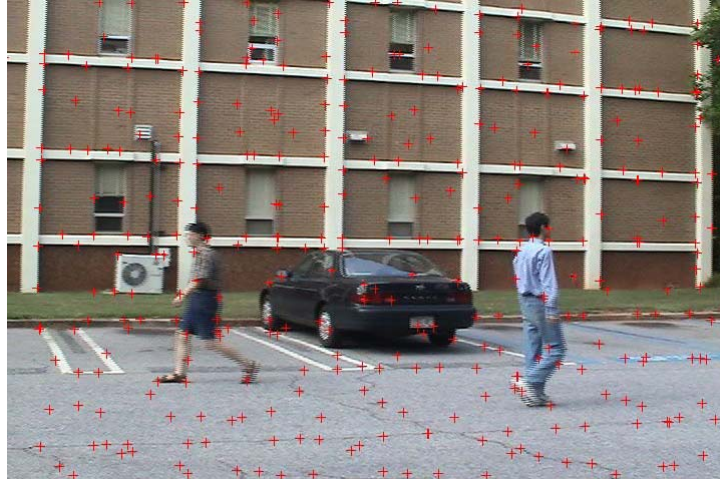
Figure 2.1: Interest points detected by the Moravec corner detector
