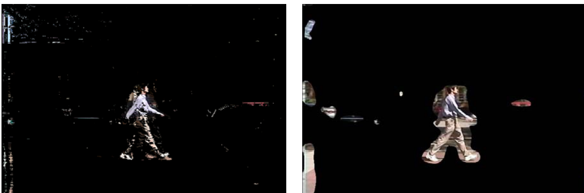
Figure 2.2: The frame on the left shows the detected regions corresponding to the moving objects prior to smoothing. The one on the right shows the detected regions corresponding to the moving objects after smoothing by a two-dimensional Gaussian filter.
