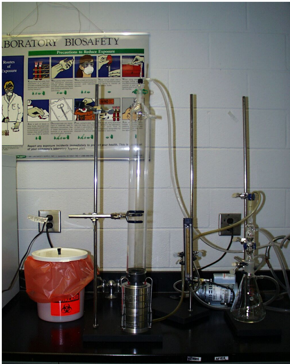
Figure 3-2. Bacterial filtration efficiency test apparatus
