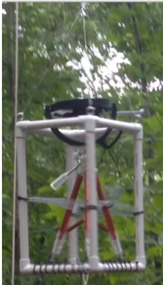
Figure 2. Camera rig for hemispherical photos of canopy. Constructed using PVC pipes, hardware cloth, and heavy duty fishing line.
