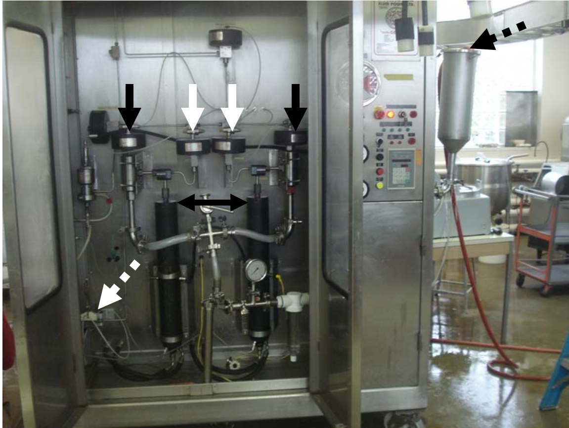
Figure 3.4 - Inside view of Stansted CFHPT system (Model nG7900, Stansted Fluid Power Ltd., Stansted, Essex, UK) with throttling valve (dashed white arrow), intensifiers (two head black arrow), inlet valves to intensifiers (black arrow), outlet valve from intensifiers (white arrow), feed inlet (dashed black arrow).
