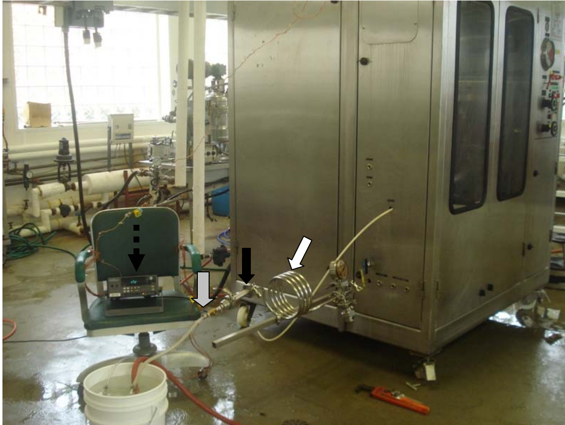
Figure 3.3- Outside view of Stansted CFHPT system (Model nG7900, Stansted Fluid Power Ltd., Stansted, Essex, UK) showing different attachments. Holding tube (white arrow), Thermocouple (black arrow), back pressure controlling valve (grey arrow), Fluke Hydra Data Bucket (PO Box 9090, Everett, WA 98206-9090), (Black dashed arrow)
