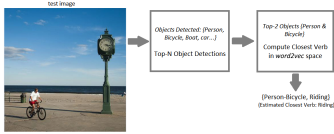
Figure 3.2: Outline of the proposed top-object detection-driven verb prediction model
